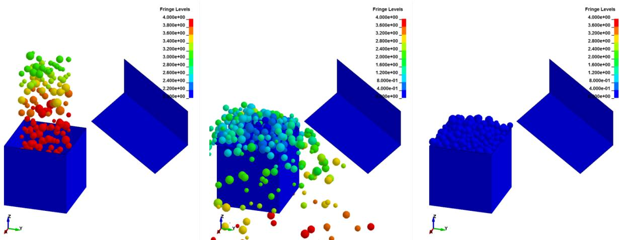
The next series of images shows the scraping process. The scraper moves across the top of the container leveling off any excess material.
