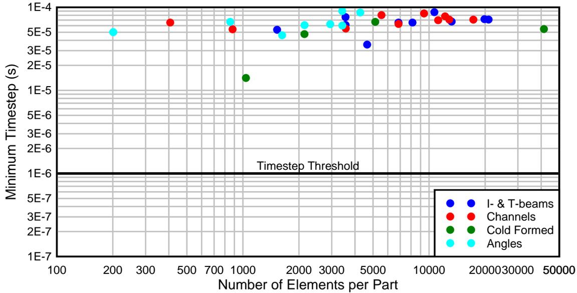
Figure 13. Minimum Time-step of Automeshed Parts
