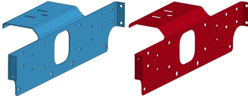
Figure 6. Uniform Thickness, Formed Part with CAD Geometry (left) and Shell Representation (right)
