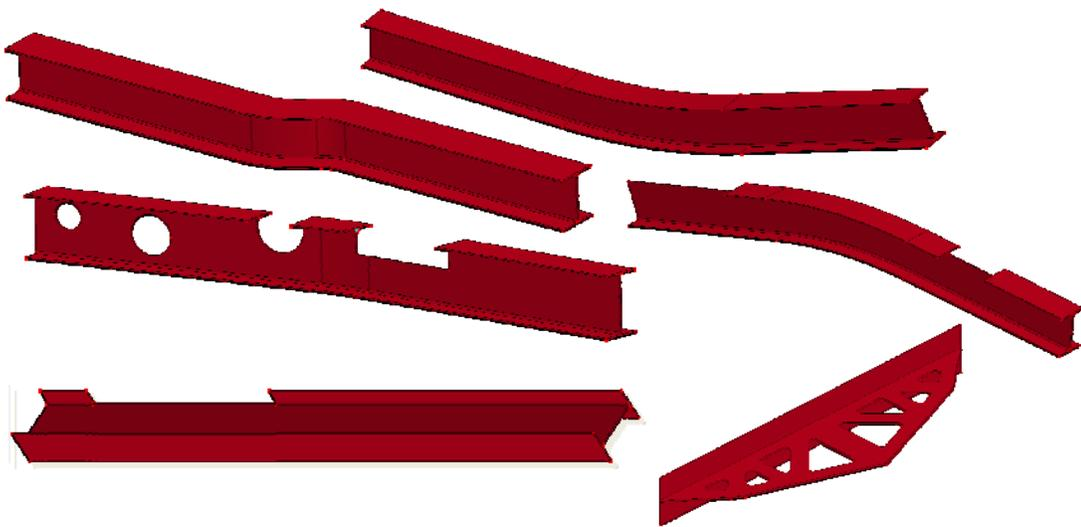
**Figure 12. I- and T-Beam Parts with Cutouts in the Web and Flange**
