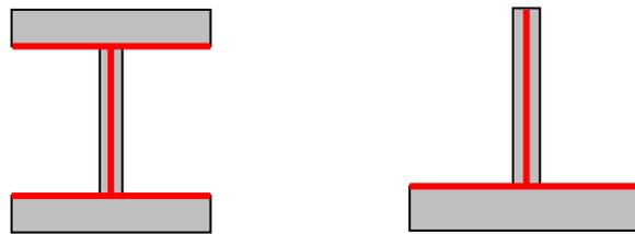
Figure 4. I-beam and T-beam Cross Section with Shell Locations shown in Red
