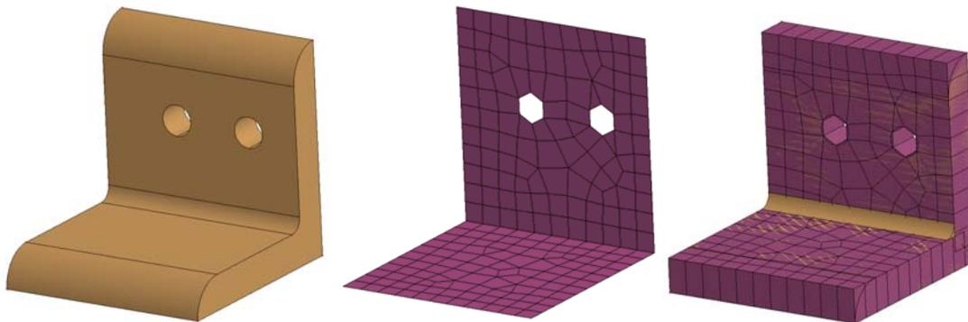
Figure 8. Angle Connection CAD geometry (left), shell presentation (middle), and overlaid mesh and CAD geometry (right)
