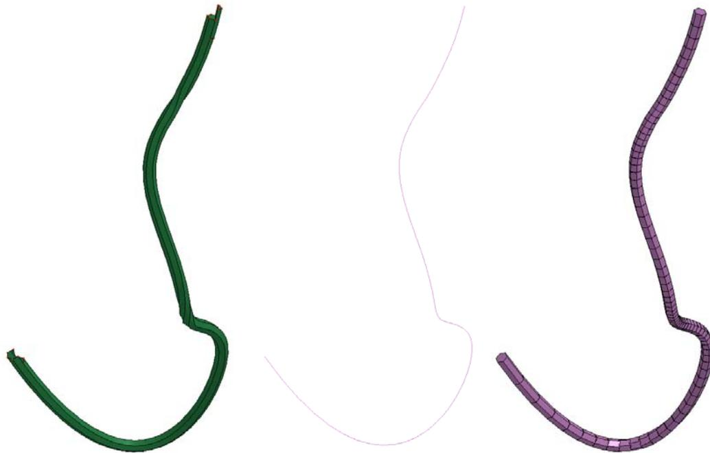
Figure 9. Complex Hexagonal Rod with CAD Geometry (left), Beam Representation (middle), and Beams with Thickness Displayed (right)
