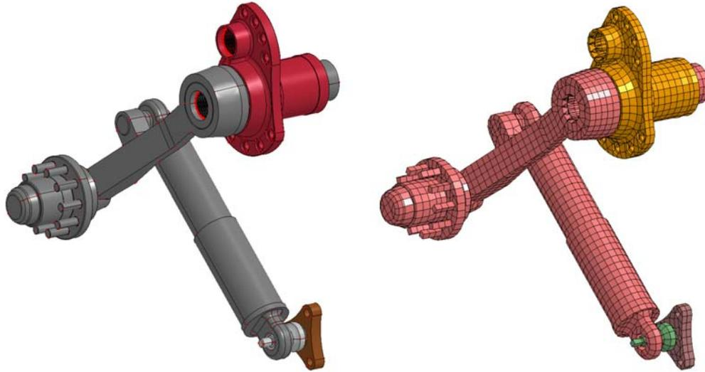
Figure 7. Surface Mesh (Rigid Parts) with CAD Geometry (left) and the Mesh Representation (right)
