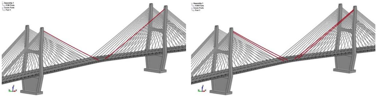
**Figure 8:** FE model with highlighted cables removed in the different cases (left) case 2 and 5 (right) case 3 and 6
