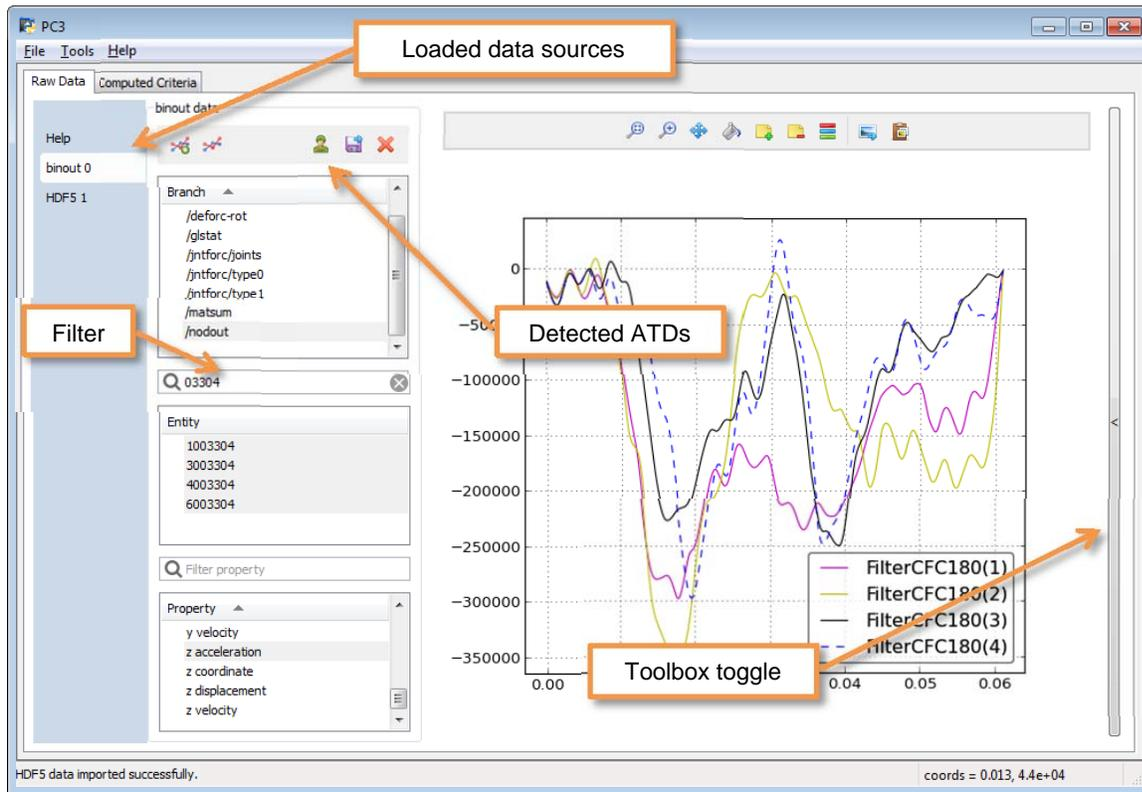
**Figure 1: PC3 GUI overview. The main menu is available on top, and below it the main panels: (a) Raw data and (b) Computed criteria. Each panel has data tables at left and plot area at right**
