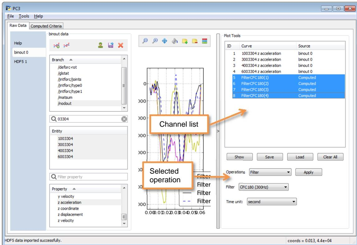
Figure 2: Toolbox open, with filtered channels shown in the plot area
