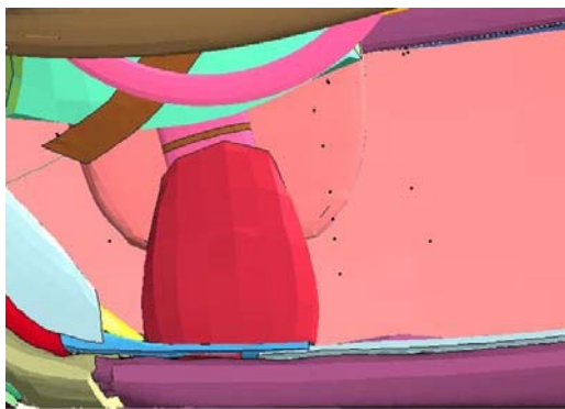
Figure 14: Head position at 0.265 sec showing roof sheet metal being driven into the cabin by the initial contact impulse. This neck position is very near the orientation at which the maximum neck force F_z occurs
