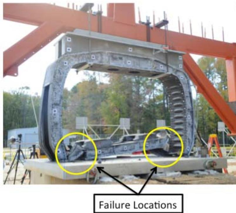
Figure 4. Frame fuselage section post-test showing failures
