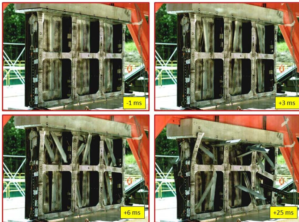
Figure 6. Northeast camera view of subfloor deformation.
