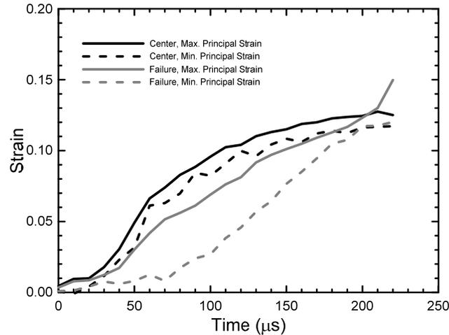
Figure 5: Maximum and minimum principle strains at the center and at the failure point.
