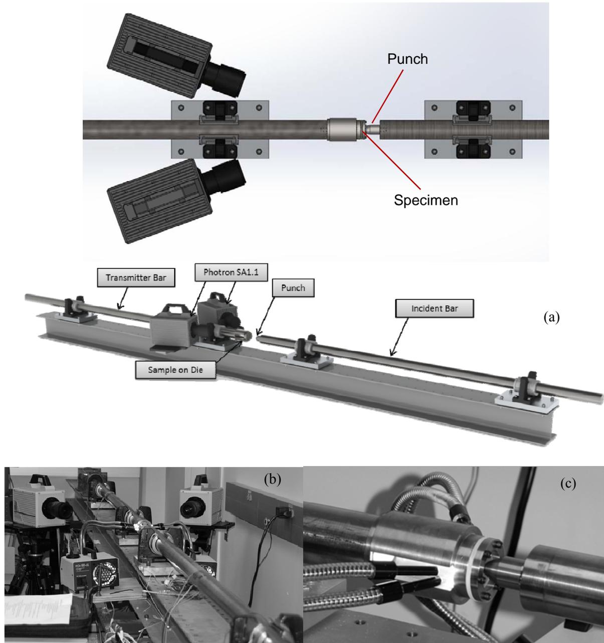
Figure 1: Experimental setup of the dynamic punch test.
