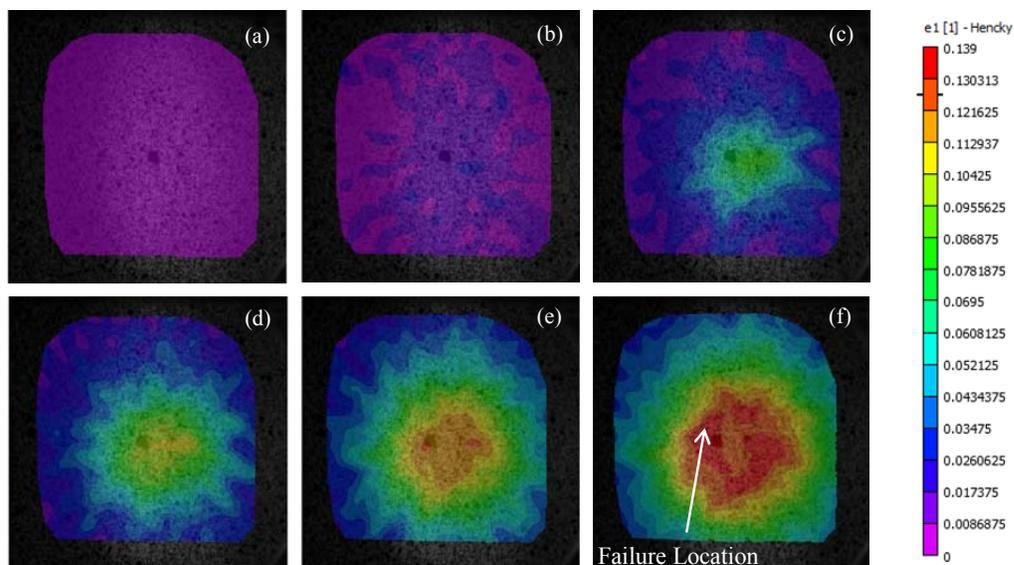
Figure 4: Maximum principal strain contours measured with 3D DIC:
