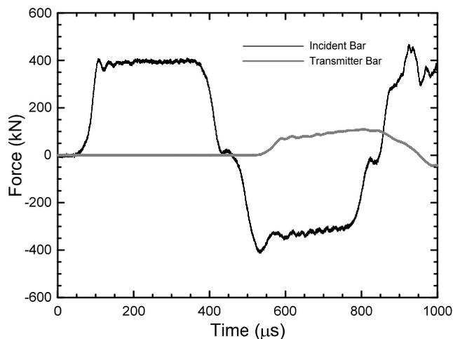
Figure 3: Waves recorded during a dynamic punch test with a hemispherical punch.
