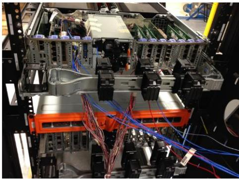
Fig.9: 2U Power9 systems with accelerometers and rosette strain gages
