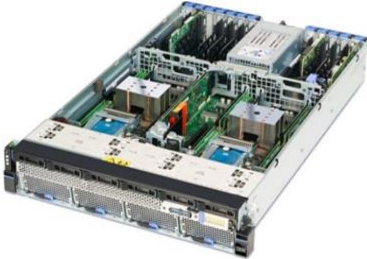
Fig.1: 2U Power9 System (Cover off)
