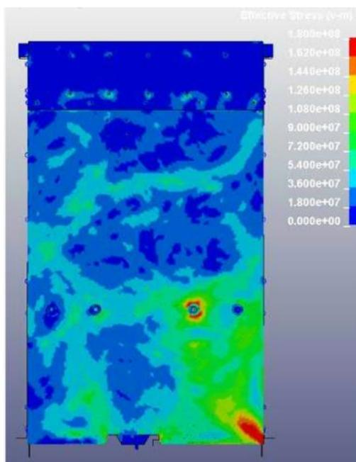
Fig.6: von Mises stress in top chassis for 2U system
