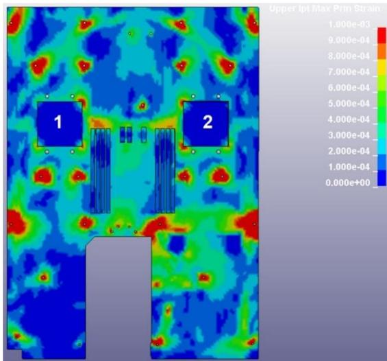
Fig.7: Upper maximum principal strain for the 2U main PCB. Locations 1 and 2 indicate the HGLAs on the PCB
