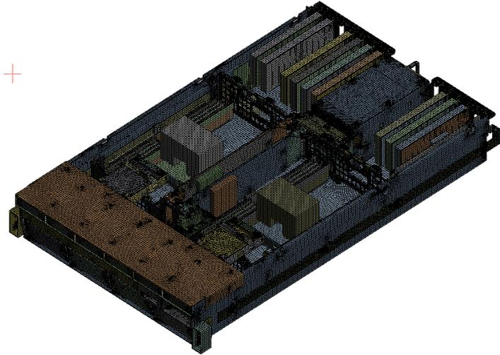
Fig.3: 2U Power9 System mesh (cover off)
