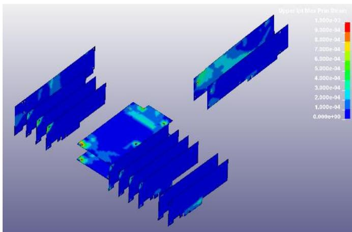
Fig.8: Upper Ipt maximum principal strain for the 2U SAS, PCIe, and power supply cards
