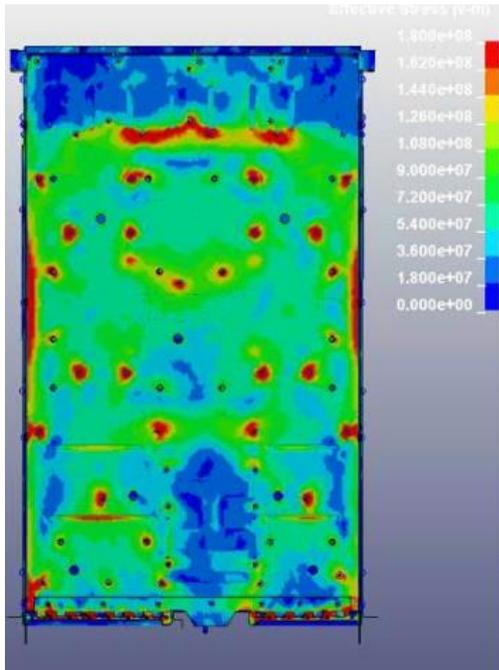
Fig.5: von Mises stress in bottom chassis for 2U system
