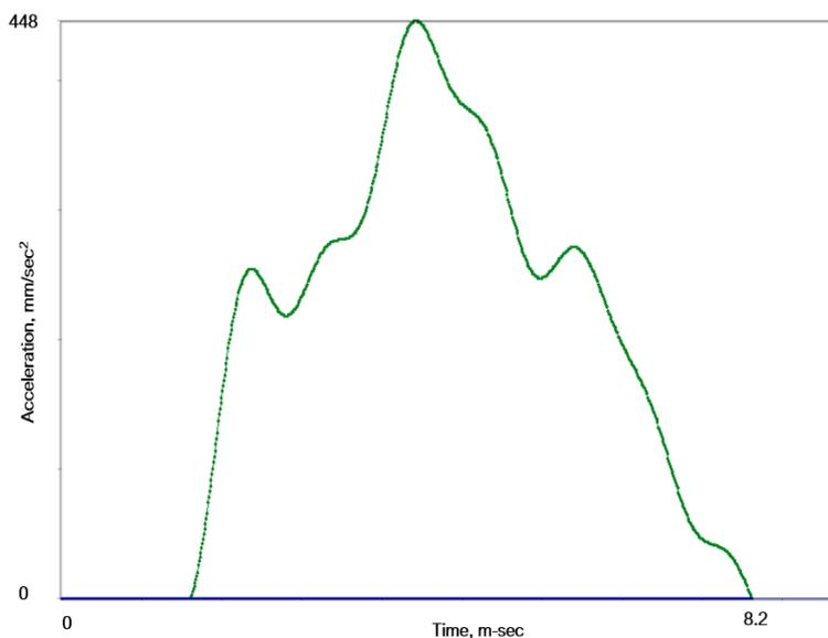
Fig.4: 70 in/s palletized rack drop profile
