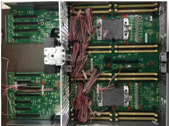
Fig.10: Main PCB with ten rosette strain gauges
