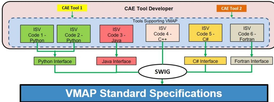
Fig.2: Figure 2: VMAP Standard implementation with other programming/scripting languages via the SWIG wrapper
