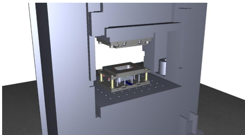
Fig. 11: Visualized simulation model of the press in ISG-virtuos
