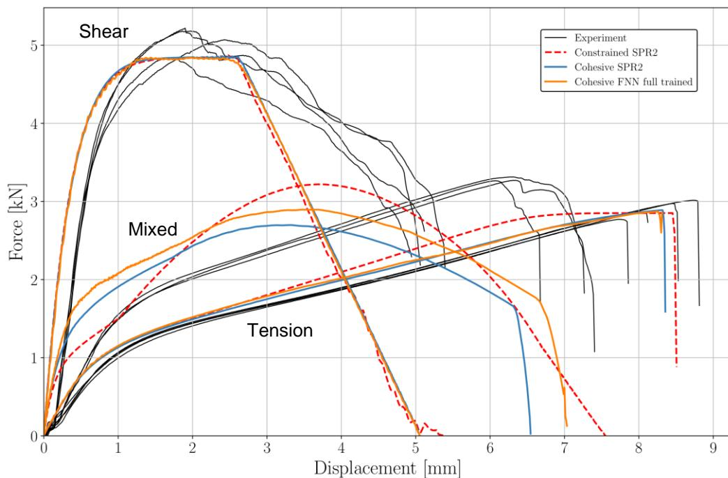
*Fig.6: Force-displacement response from crosstest under tensile, mixed and shear loading; simulation with **\*CONSTRAINED\_SPR2**, SPR2 model as cohesive element and NN model as cohesive element*
