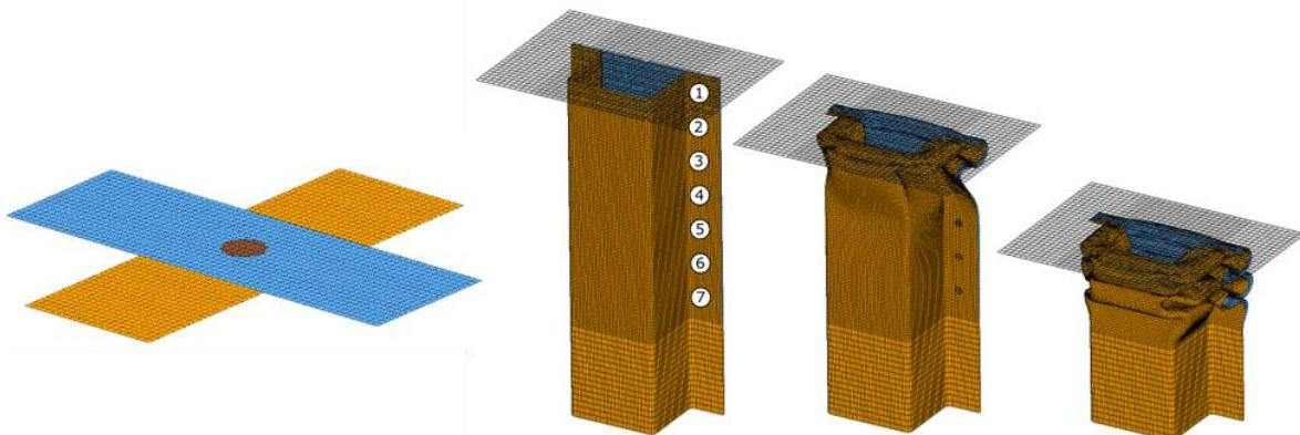
Fig.5: Crosstest for single unit test (left) and crashbox with joint numbering (right)
