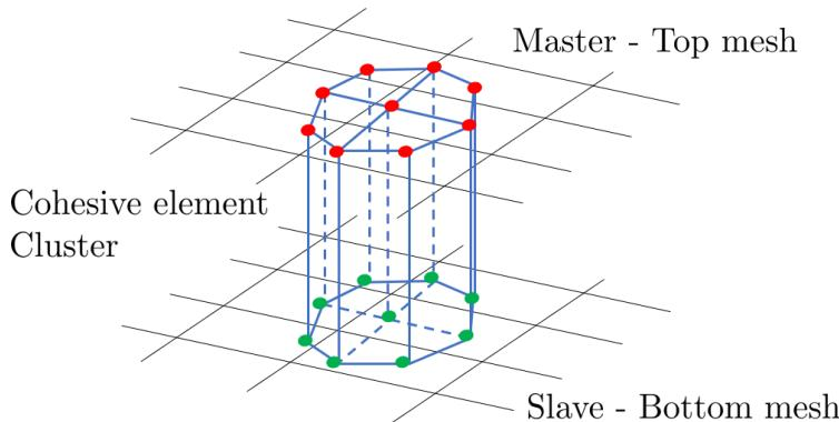
Fig.1: Large scale mesh with cluster of four cohesive elements representing joint
