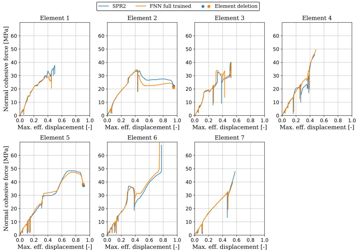
*Fig.8: Local response cohesive element 1-7; normal traction component over damage measure; failure/deletion of element 2 and 5*
