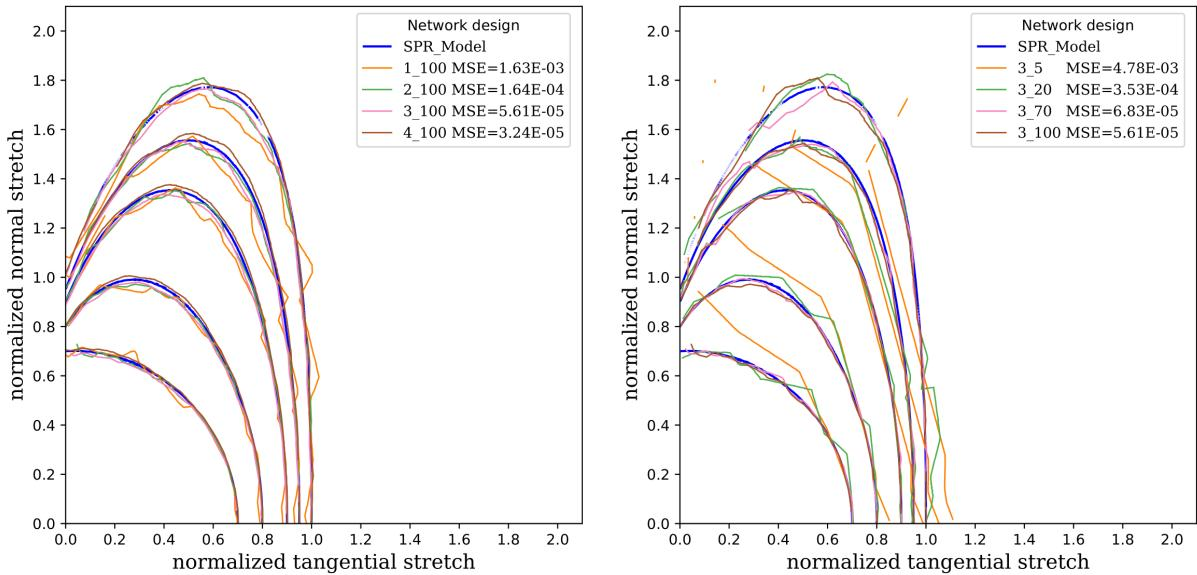
Fig.4: Contour plots with different levels of damage: 100 nodes and one to four hidden layers (left), three hidden layers and 5, 20, 70, 100 nodes (right)
