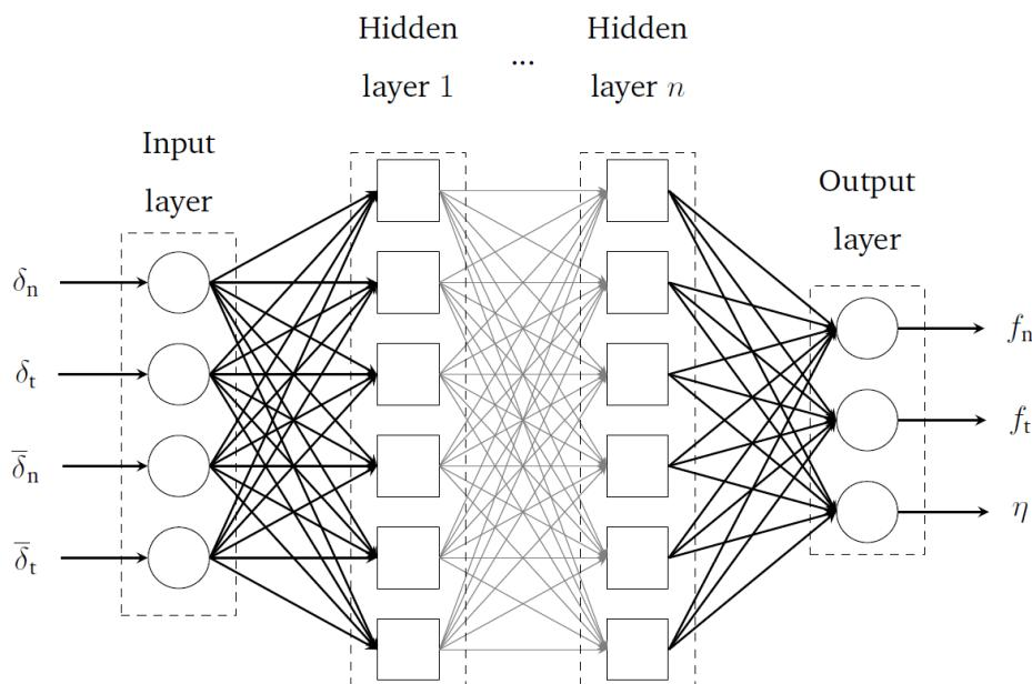
Fig.2: Fully connected feedforward NN; four input variables (stretches, stretch histories) and three output variables (forces/tractions, damage)
