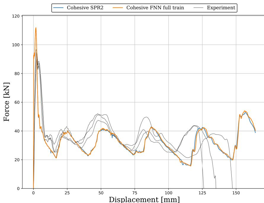
*Fig.7: Global force-displacement response component simulation*
