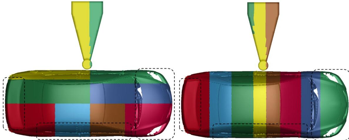
Fig.19: Model decomposition using RCB (left) and `CONTROL_MPP_DECOMPOSITION_AUTO-MATIC` (right) over 8 CPUs. The rectangular highlights reflect the location of the reduced parts.
