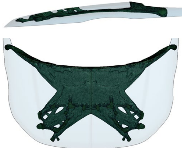
Fig. 6: Optimized structure of the inner panel of the engine hood for impact and static load cases
