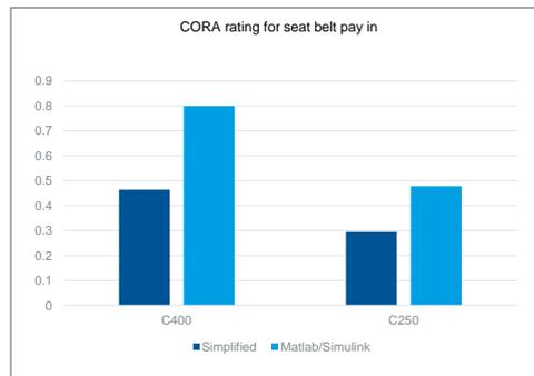
Fig.5: CORA rating of webbing pay in for  $C_{400}$  configuration (left) and  $C_{250}$  configuration (right) for simplified (dark blue) and Matlab/Simulink (light blue) MBPPT modelling methods.
