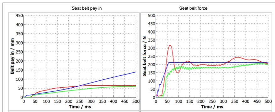
Fig.3: Webbing pay-in (left) and seat belt force level (right) for  $C_{250}$  configuration. The simplified MBPPT model in blue, the Matlab/Simulink model in green and the physical test data in red.
