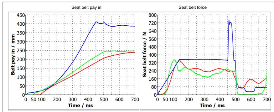
Fig.2: Webbing pay in (left) and seat belt force level (right) for  $C_{400}$  configuration. The simplified MBPPT model in blue, the Matlab/Simulink model in green and the physical test data in red.
