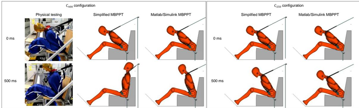
Fig.4: Kinematic comparison of  $C_{400}$  (left) and  $C_{250}$  (right) for both modelling methods showing the initial position (top row) and position at 500 ms (bottom row). For  $C_{400}$  the physical testing is given as reference.
