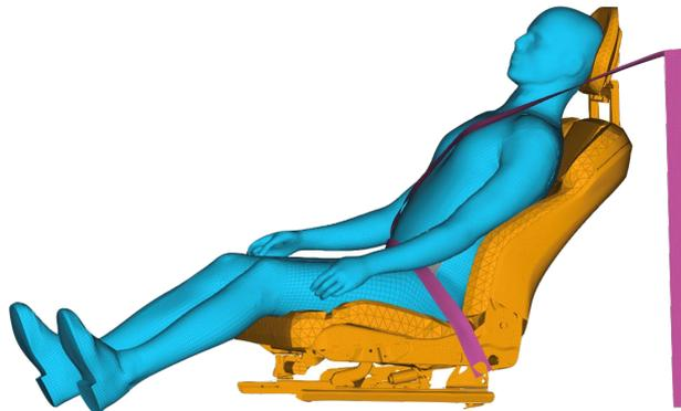
*Fig.6: Positioning the GHBMCM50 in a reclined position, together with seat kinematics and restraining*
