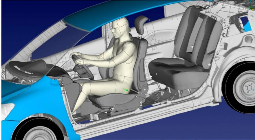
*Fig.4: Interactive positioning of an HBM*
