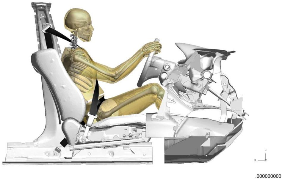
Fig.11: Front sled impact model with GHBMCM50-O v5.1.1 occupant model positioned in driver seat
