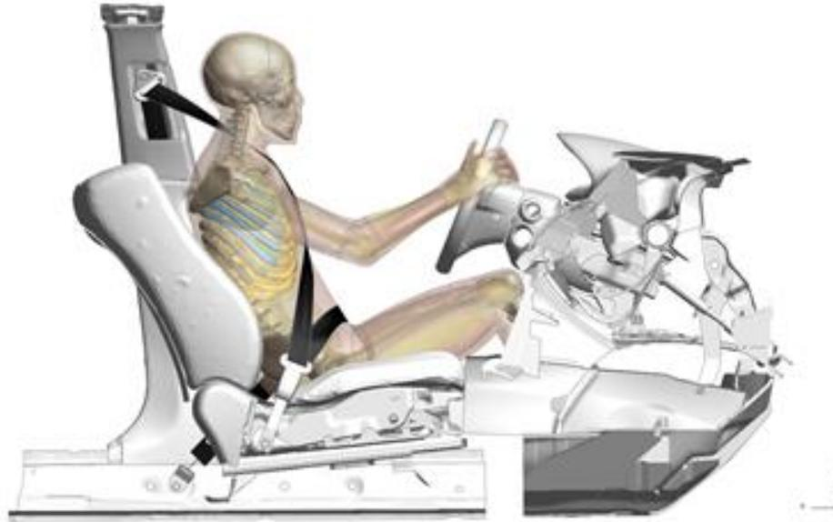
Fig.9: Front sled impact model with THUMS AM50-O v4.1 occupant model positioned in driver seat
