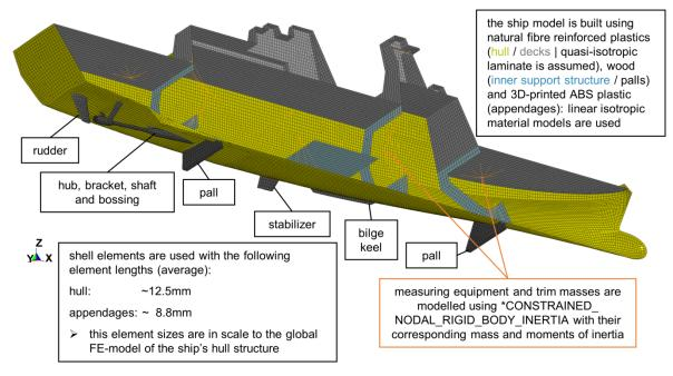
Fig.10: FE-model of ship model used for model tests of sideways launching process
