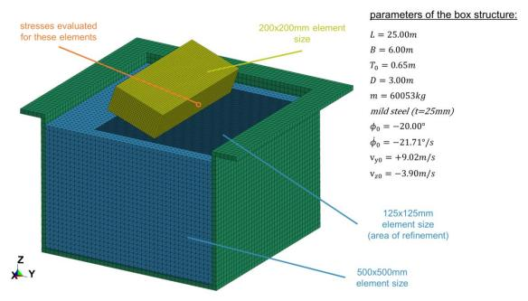
*Fig.4:* FE-model of a box structure impacting the water surface used for investigation of relevant parameters for ALE-approach
