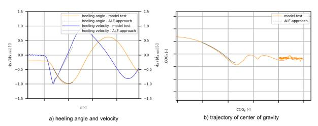
Fig.12: Results of the ALE-approach compared to model tests of a sideways launching process movement of the ship
