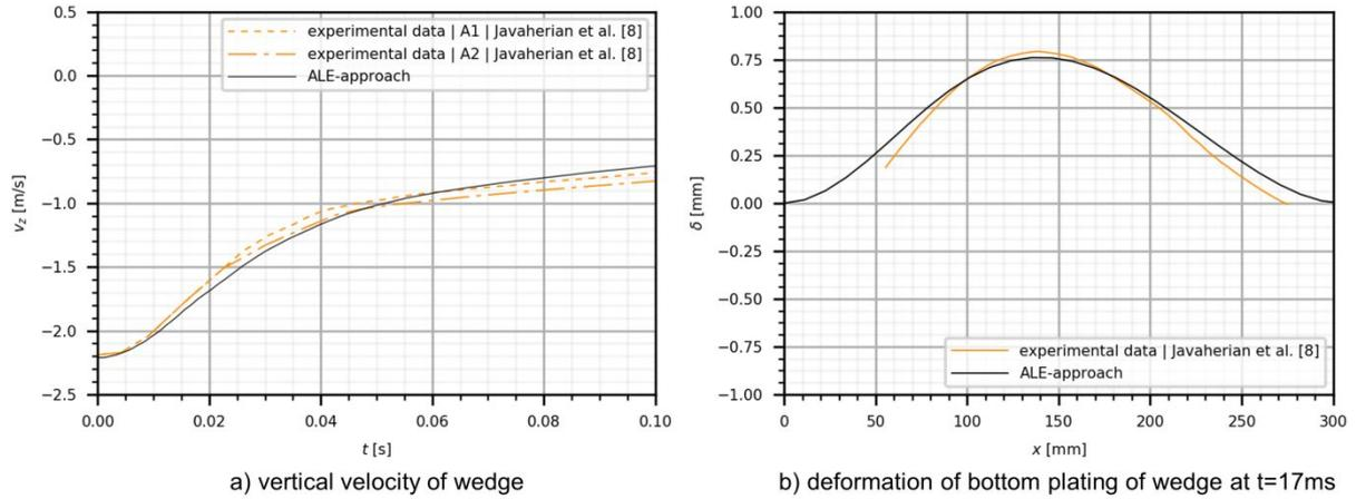
Fig.2: Kinematics of a wedge during slamming experiments conducted by Javaherian et al. [8]
