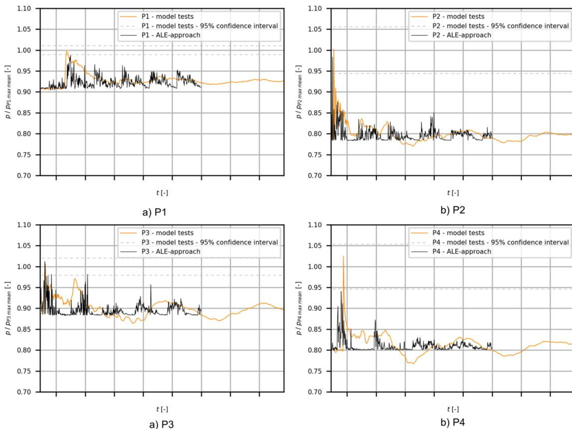
Fig.11: Results of the ALE-approach compared to model tests of a sideways launching process – pressure-time histories at different points of the ship hull
