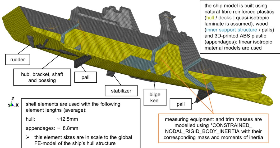
Fig.10: FE-model of ship model used for model tests of sideways launching process
