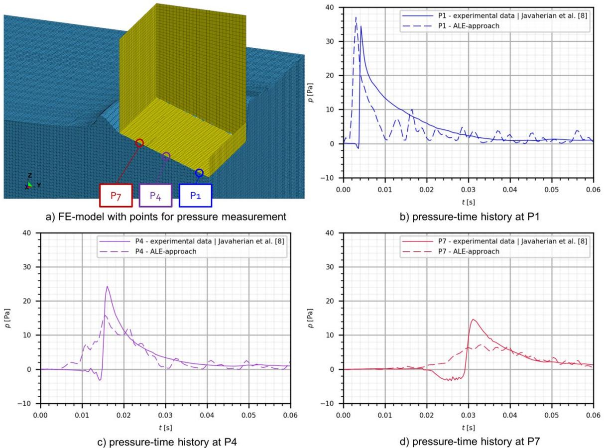
Fig. 1: Pressure-time histories of slamming experiments conducted by Javaherian et al. [8]
