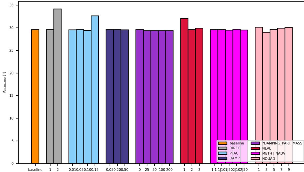
Fig.8: Influence of different parameters on the maximum heeling angle of the box structure
