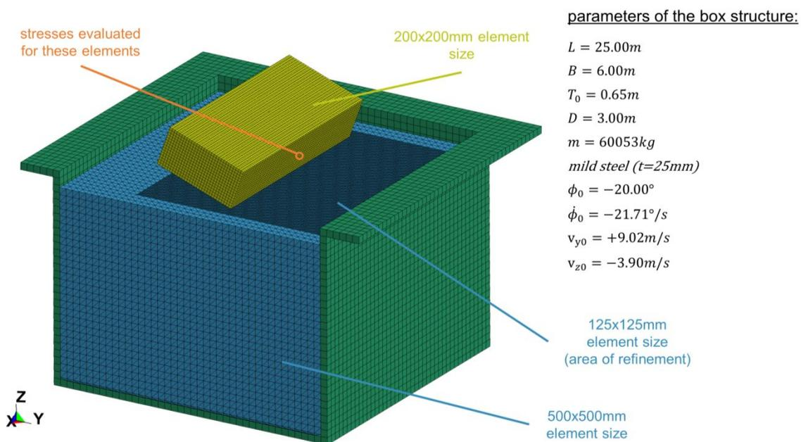
Fig.4: FE-model of a box structure impacting the water surface used for investigation of relevant parameters for ALE-approach
