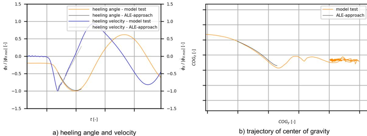
Fig.12: Results of the ALE-approach compared to model tests of a sideways launching process - movement of the ship
