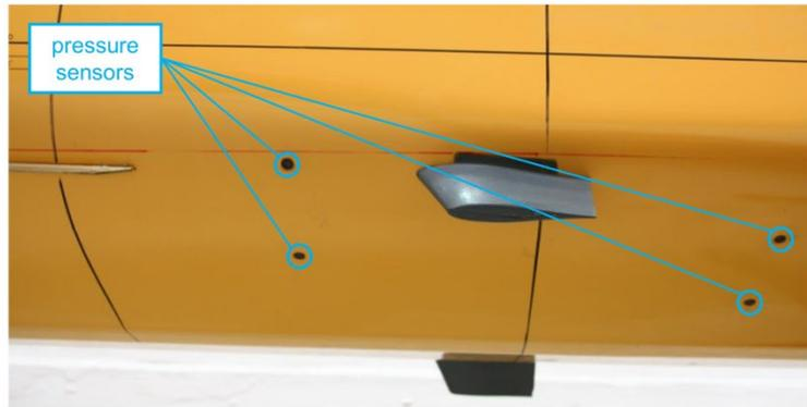
b) measurement equipment used during model tests at ship model basin
