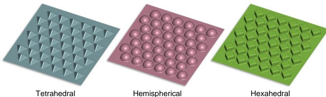
Fig.2: Geometry of three core panels
