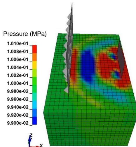
Fig.5: Sound pressure distribution example (tetrahedral core panel, 400 Hz)
