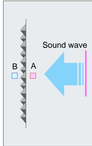
Fig.4: Position of ALE elements that output sound pressure (top view)
