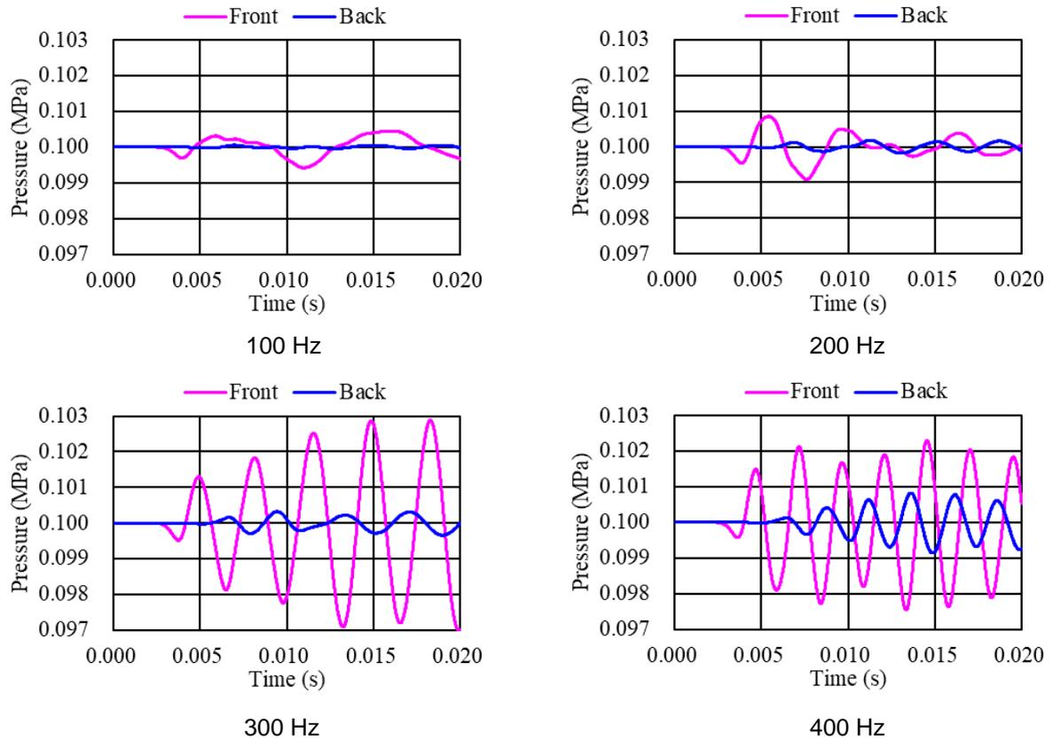
Fig.7: Pressure history for hemispherical core panel
