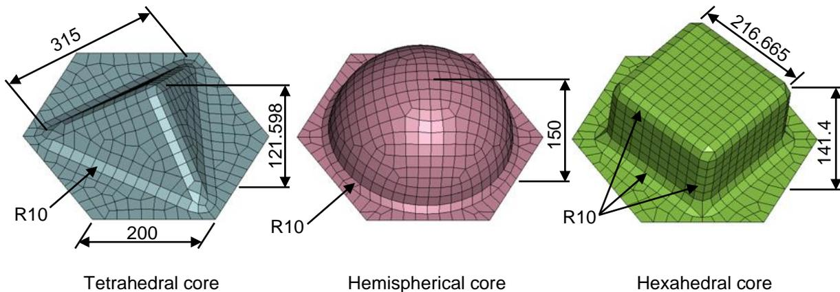
Fig.1: Core geometries to be compared (length unit : mm)
