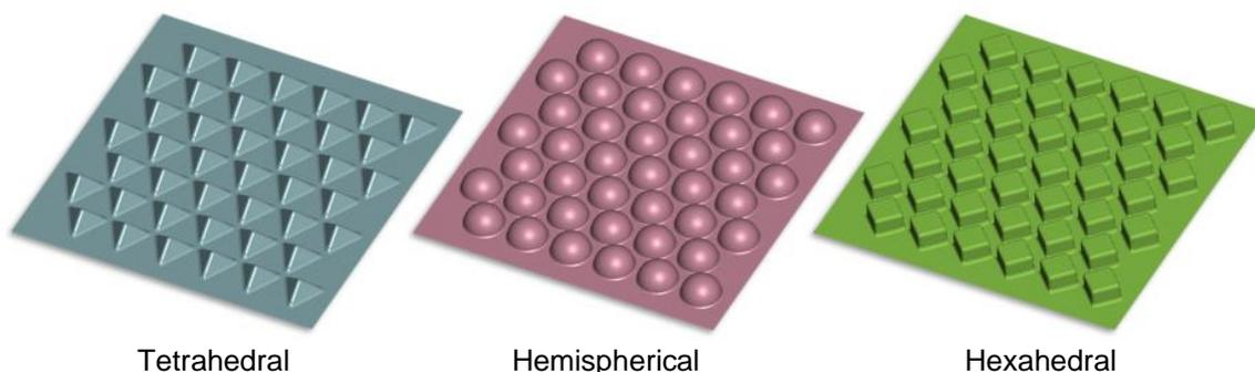
Fig.2: Geometry of three core panels
