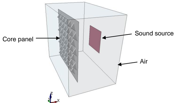
Fig.3: Model configuration for acoustic analysis
