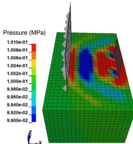
Fig.5: Sound pressure distribution example (tetrahedral core panel, 400 Hz)
