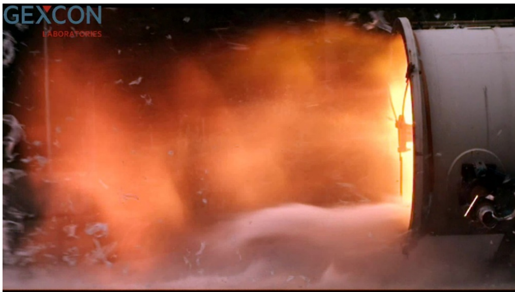
Fig.2: Example of a hydrogen explosion large scale experiments on Gexcon test site
