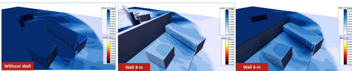
Fig. 8: Comparison of base case (left) and protective walls simulations (middle and right)
