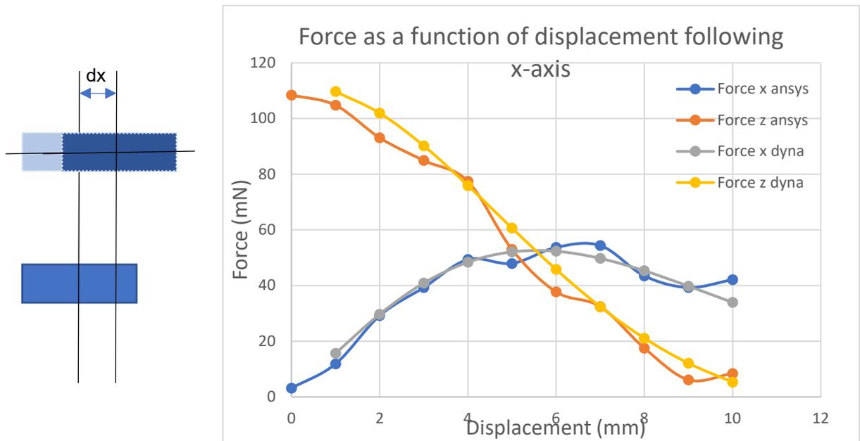
Fig. 5 Magnetic force versus displacement following x-axis
