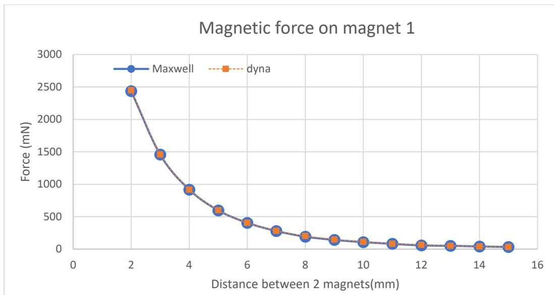
Fig. 1 Magnetic force versus distance between 2 magnets in linear case
