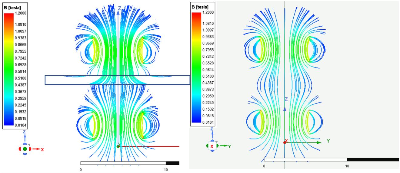
Fig. 7 Magnetic field streamline with (left) and without (right) steel plate
