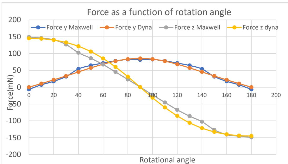
Fig. 4 Magnetic force versus rotation angle in nonlinear case
