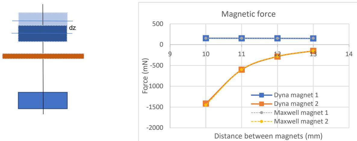
Fig. 6 Magnetic force in magnet 1 and 2 obtained by Dyna and Maxwell
