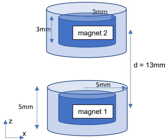
The ANSYS Maxwell solver generates a tetrahedral mesh (for the magnets and the surrounding air) while LS-DYNA generates a hexahedral mesh (of the magnets only). In the next section of comparison, one magnet will be moved along the z-axis, x-axis, or rotated around an axis.
