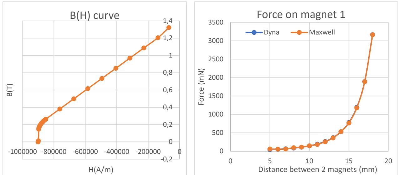
Fig. 2 BH curve (left) and magnetic force versus distance between 2 magnets (right)
