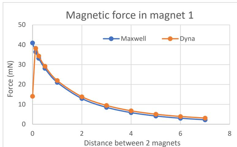
Fig. 8 Magnetic force in magnet 1 as a function of distance between 2 magnets
