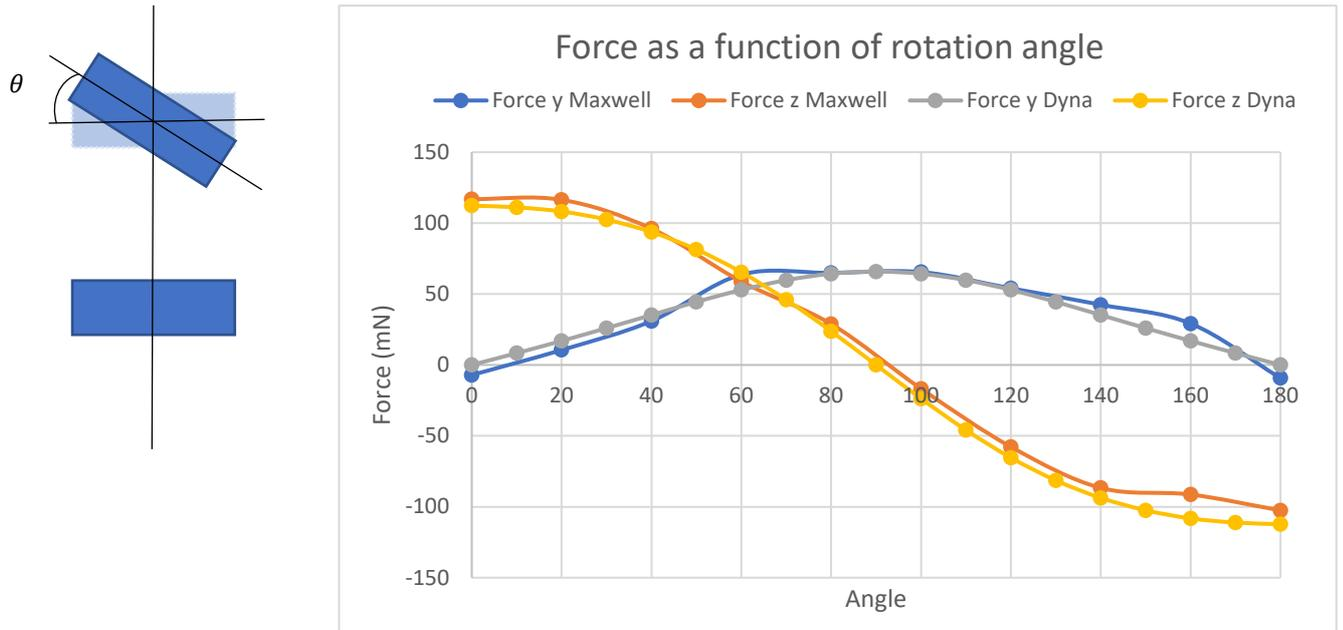
Fig. 3 Magnetic force versus rotation angle in linear case
