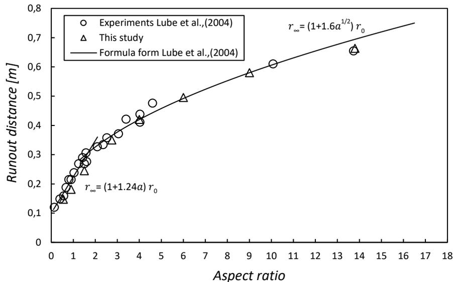
Figure 3: Comparison of final runout distance between SPH simulations and experiments in [1]
