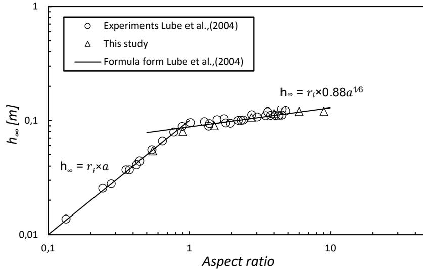
Figure 4: Comparison of final deposit height between SPH simulations and experiments in [1]
