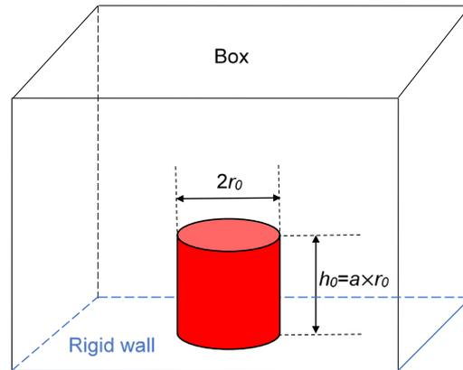
Figure 1: Initial SPH-based granular column model in LS-DYNA
