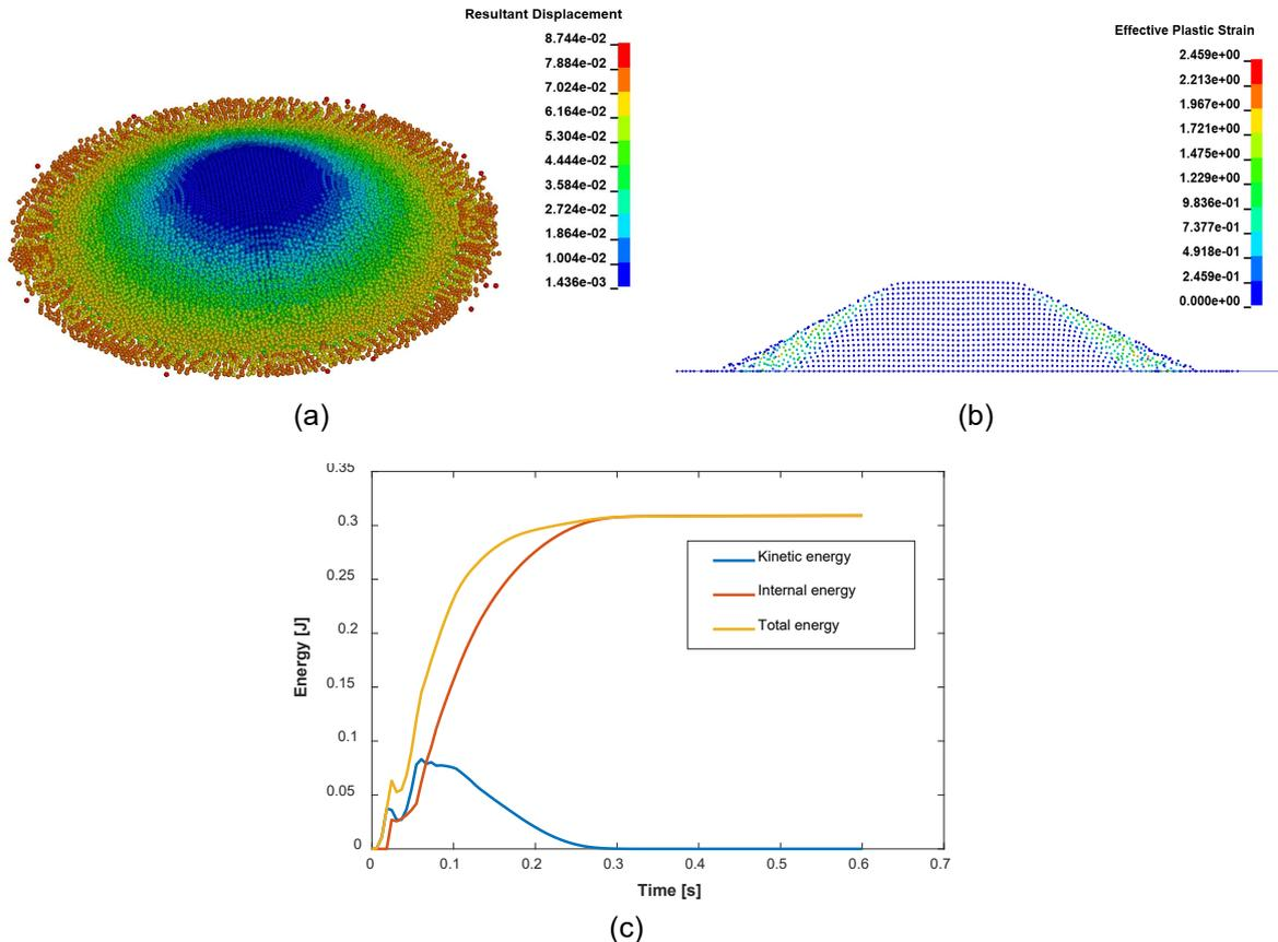
Figure 5: Additional results ( $a=0.55$ ) (a) resultant displacement; (b) plastic strain; (c) energy variation with time
