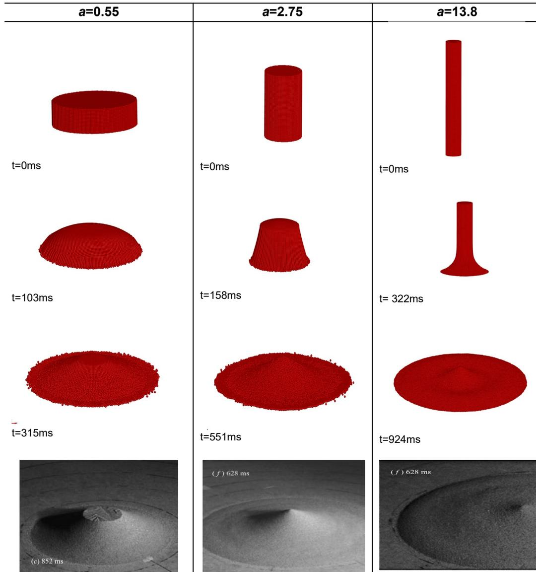
Figure 2: Granular column collapse evolution at various time points observed in three columns with representative aspect ratios (small to large from left to right, colored images) and final experimental collapse patterns reported in [1] (grey images).
