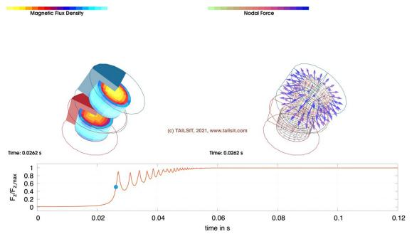
*Fig.1:* Two snapping magnets coated by non-magnetic material: magnetic flux density (left), nodal forces (right) and the total attracting force component (bottom)
