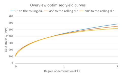
Fig. 5: Optimised strain curves w.r.t. the rolling direction using the Hockett & Sherby approach
