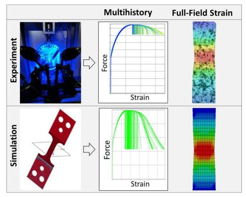
Fig. 2: Overview Full-Field-Calibration FFC approach
