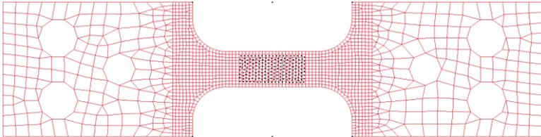
Fig. 1: Aligned experimental strain field (black) in the simulation model (red)
