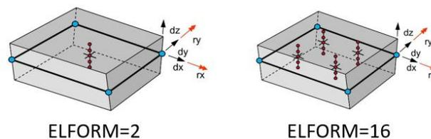
Fig. 3: Comparison of Shell element formulation 2 (left) and Shell element formulation 16 (right) [13]
