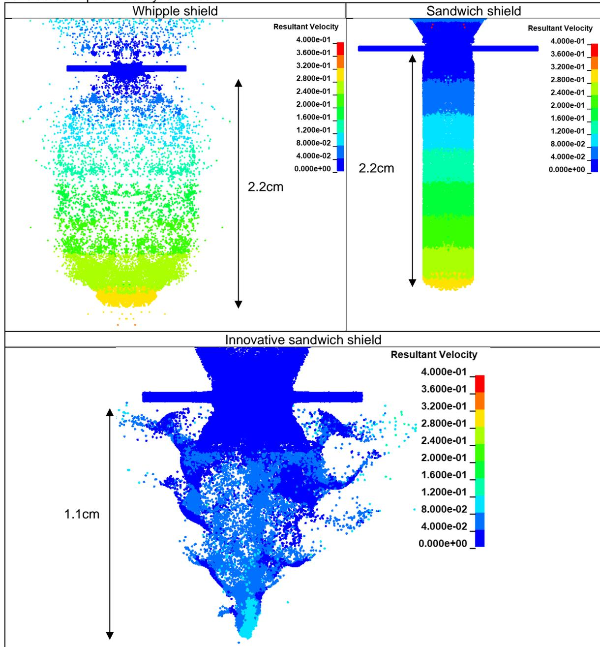
Fig.9: Debris clouds generated by a 1mm diameter impactor at 4km/s against a Whipple shield, a sandwich one and the innovative one
