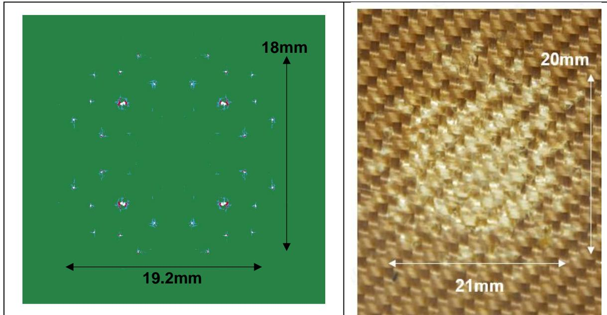
Fig.4: Zylon sheet profile with reflections of the quarter model (rear view, 6km/s)
