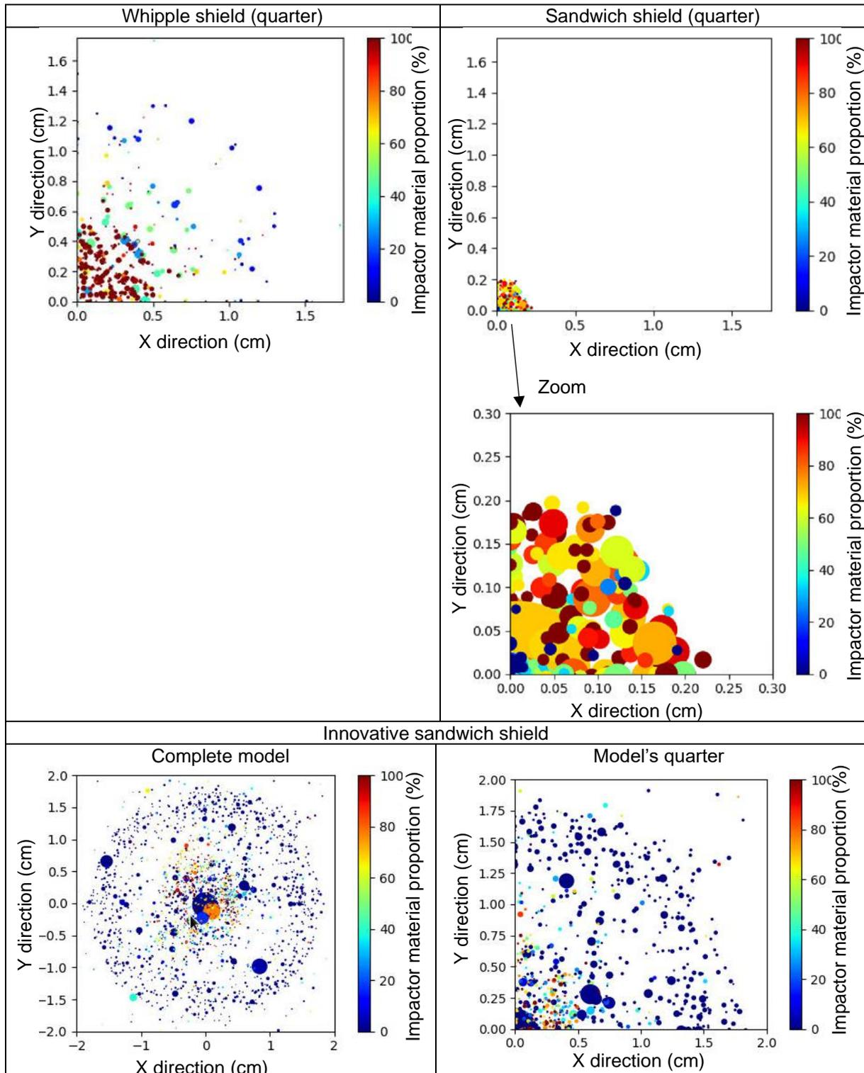
Fig.11: Visualisation of the impactor material proportion of the projected debris cloud for the Whipple shield, the sandwich shield and the innovative structure - 4km/s impact (top view)
