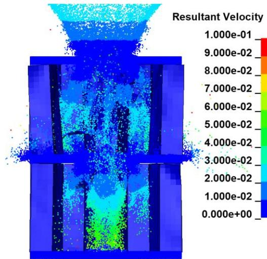
Fig.7: Sandwich shield behaviour with a 0.4mm intermediate sheet impacted by a 1mm diameter debris at 4km/s (sectional view). Velocities in cm/ $\mu$ s
