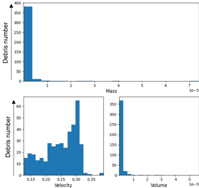
Fig.3: Mass, velocity and volume debris number repartitions - Aluminium 4km/s impact (quarter model, units: g, cm,  $\mu$ s)
