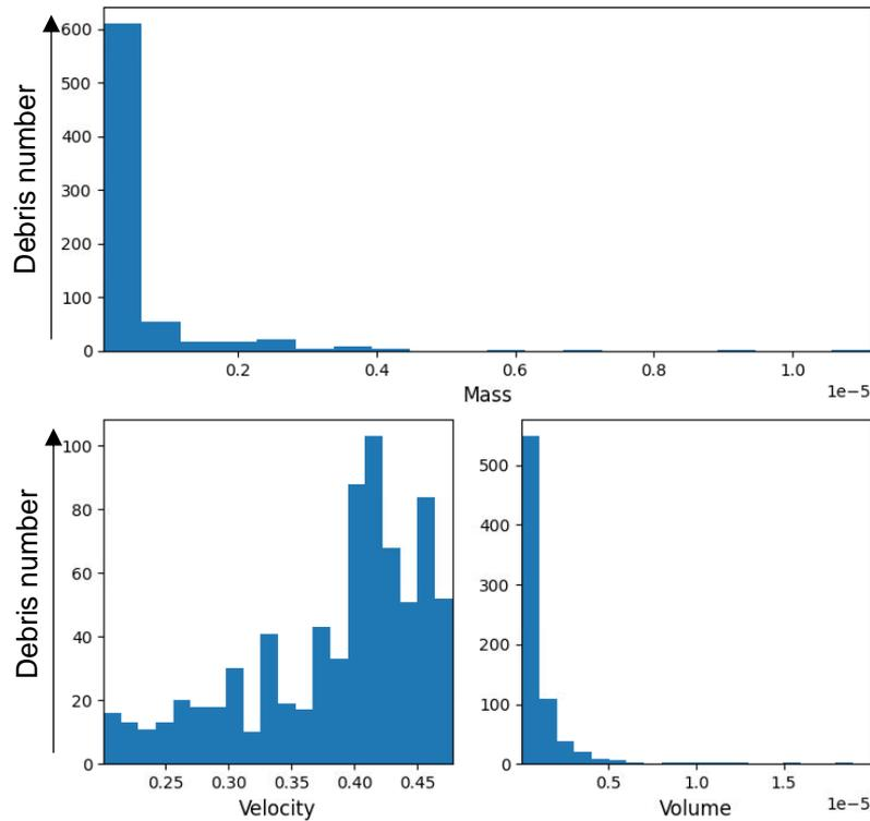
Fig.6: Mass, velocity and volume debris number repartitions - Aluminium 6km/s impact (quarter model, units: g, cm,  $\mu$ s)
