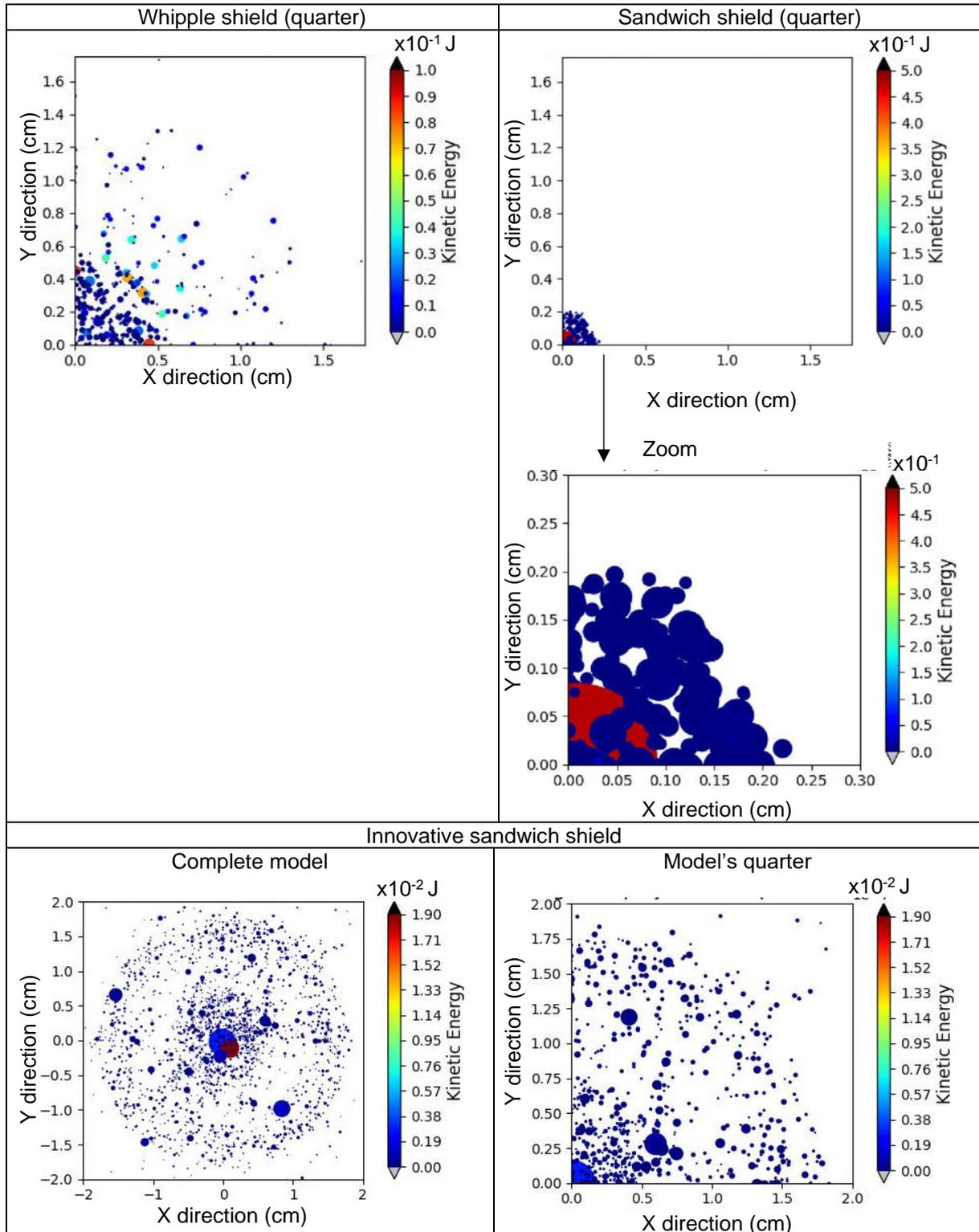
Fig.10: Visualisation of the kinetic energy of the projected debris cloud for the Whipple shield, the sandwich shield and the innovative structure - 4km/s impact (top view)
