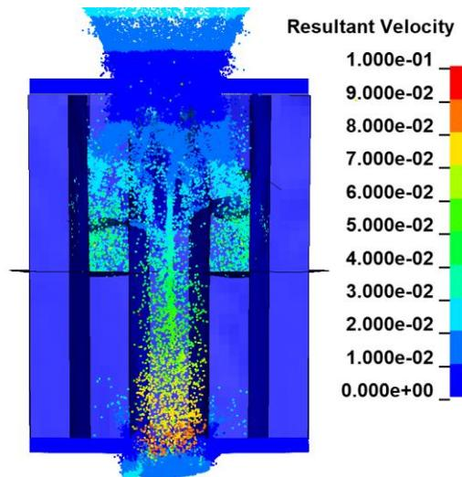
Fig.8: Sandwich shield behaviour with a 25 $\mu$ m intermediate sheet impacted by a 1mm diameter debris at 4km/s (sectional view). Velocities in cm/ $\mu$ s
