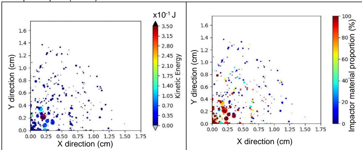
Fig.2: Visualisation of energy and impactor material proportion of the projected debris cloud - CFRP 4km/s impact (top view of a quarter model)
