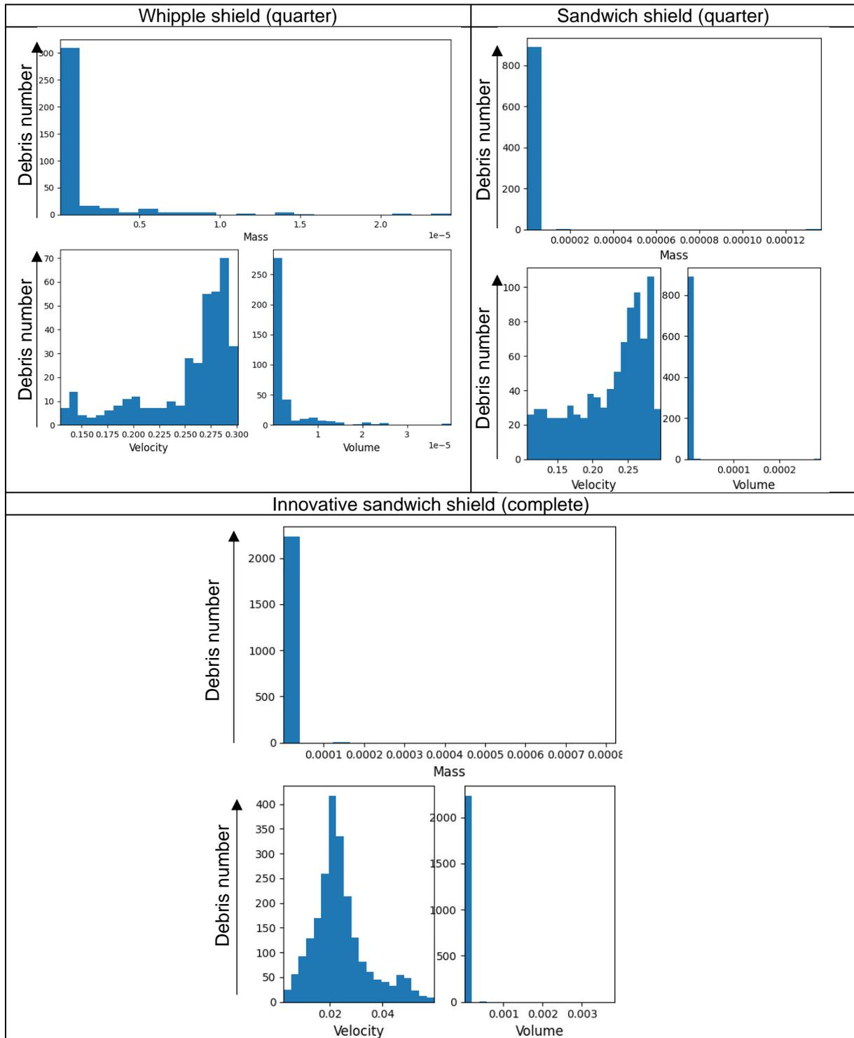
Fig.12: Mass, velocity and volume repartitions for the Whipple shield, the sandwich shield and the innovative structure - 4km/s impact (units: g, cm,  $\mu$ s)
