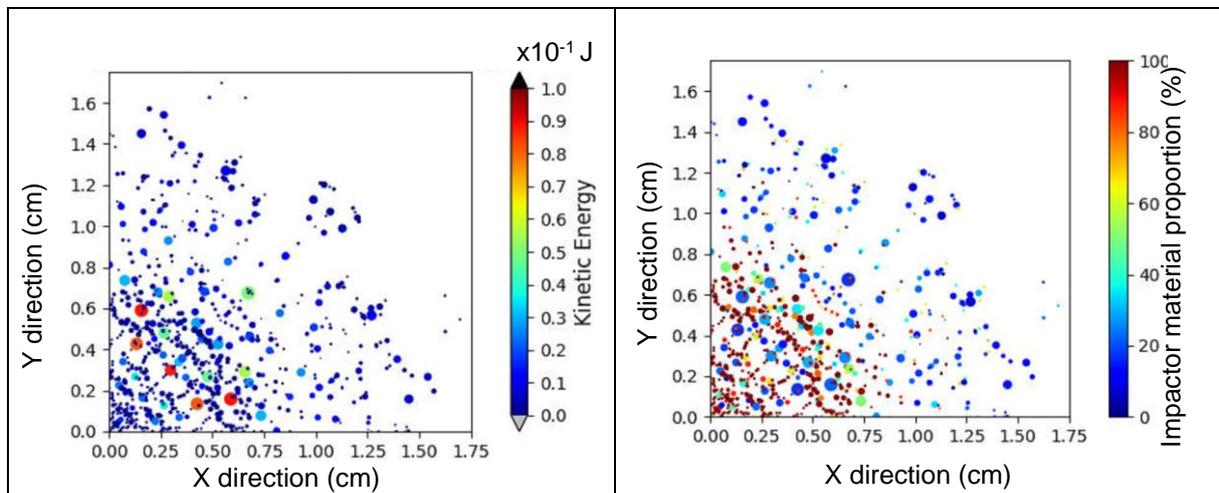
Fig.5: Visualisation of energy and impactor material proportion of the projected debris cloud - Aluminium 6km/s impact (top view of a quarter model)
