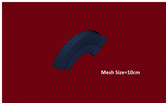
Fig.2: Finite element model of the target building- element size 10cm.
