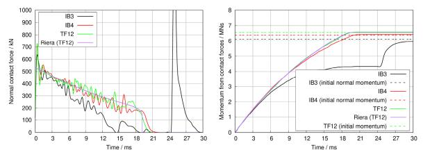
Fig.6: Comparison of numerical contact forces and momentum transfer for tests IB3, IB4 and TF12.
