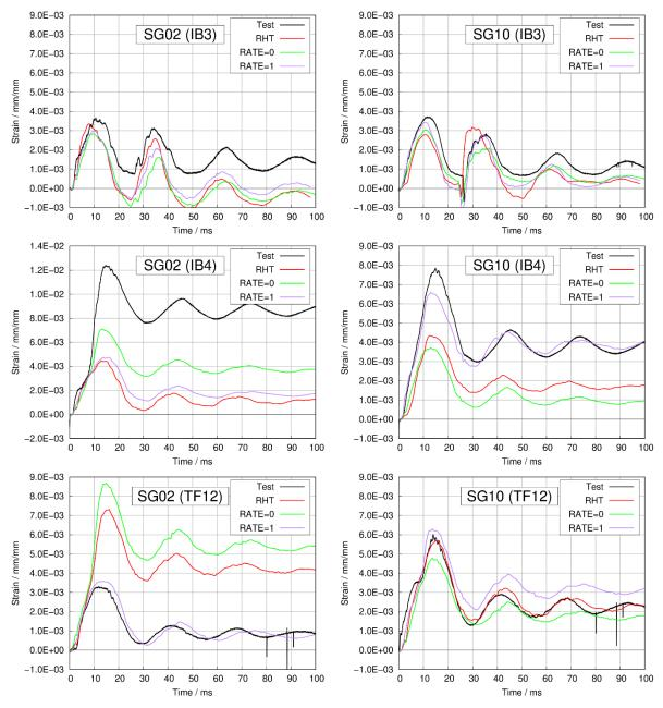
Fig. 10: Reinforcement strains at selected sensor locations for IB3, IB4 and TF12.
