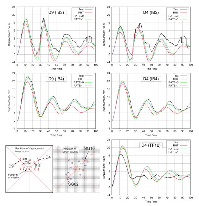
*Fig.9:* Calculated and measured back face slab displacements at selected sensor locations for IB3, IB4 and TF12.
