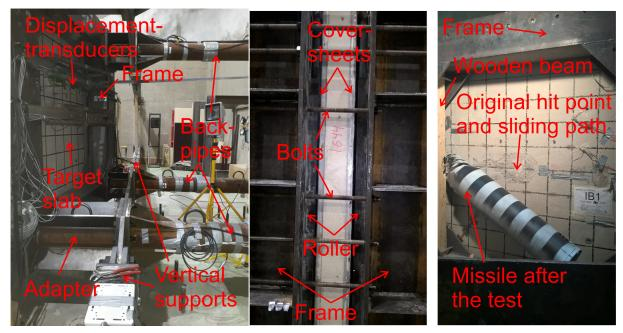
Fig.1: Details on experimental set-up on rear (left), side (middle) and front face (right) for IB1.
