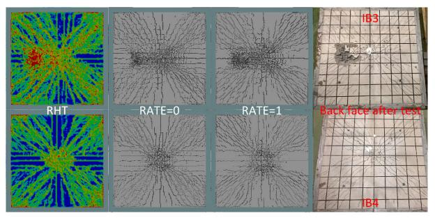
Fig.7: Comparison of back face slab damage after 100 ms and test results of tests IB3 and IB4.
