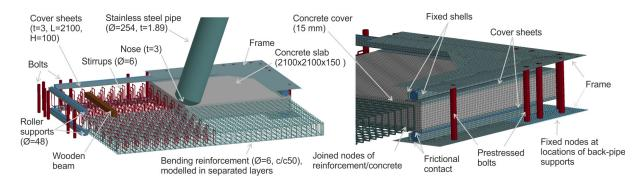
Fig.2: Details of an LS-DYNA model used for inclined soft impact simulations (dimensions in mm).
