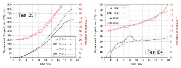
Fig.4: Comparison of measured and simulated kinematic data of the missiles in IB3 and IB4.
