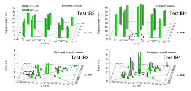
Fig.11: Comparison of measured and simulated spatial slab displacement and reinforcement strain distributions after 15 ms.
