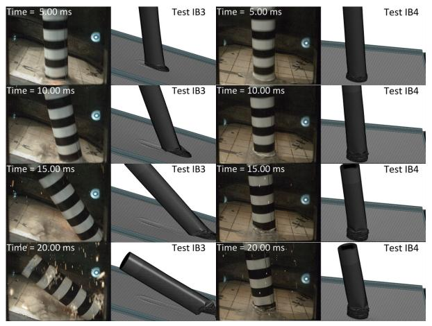
Fig.3: Comparison of missile behaviour in tests and simulations for test cases IB3 and IB4.
