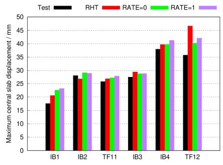
Fig.8: Comparison of maximum central slab displacements in the first cycle.
