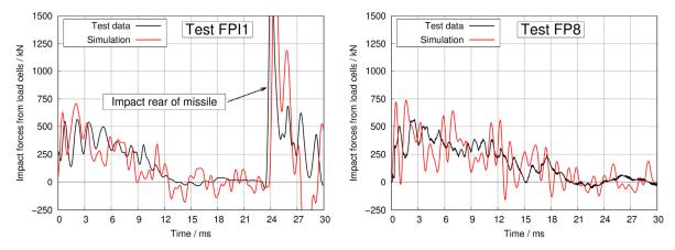
Fig.5: Comparison of numerical results on force plate test FPI1 and FP8 simulations with test data.
