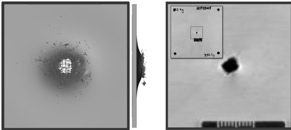
Fig.4: Rear wall damage: simulation (grid cells: 1x1 mm) vs. NASA experiment (HITF 9005, [18])
