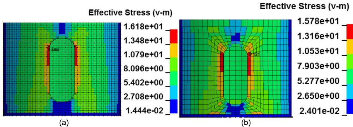
Fig. 19: The effective stress RMS (a) IGA; (b) FEA.
