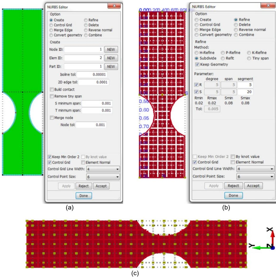
Fig.2: The mesh model construction (a) Rough mesh model; (b) Mesh refinement; (c) Final mesh model.
