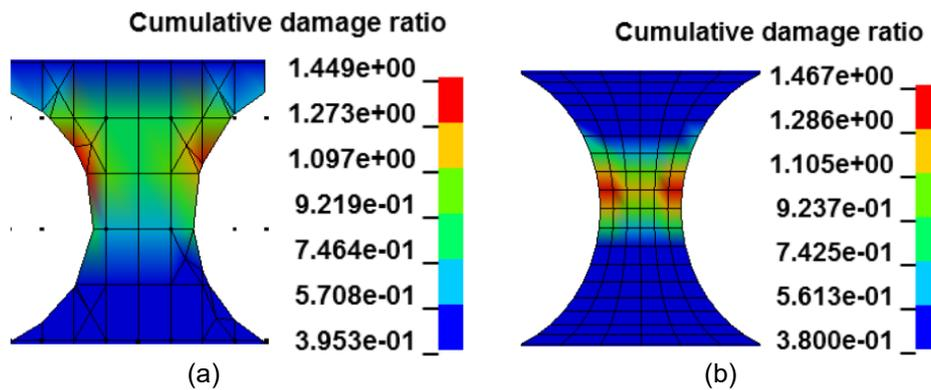
Fig. 14: The cumulative damage ratio (a) IGA; (b) FEA.
