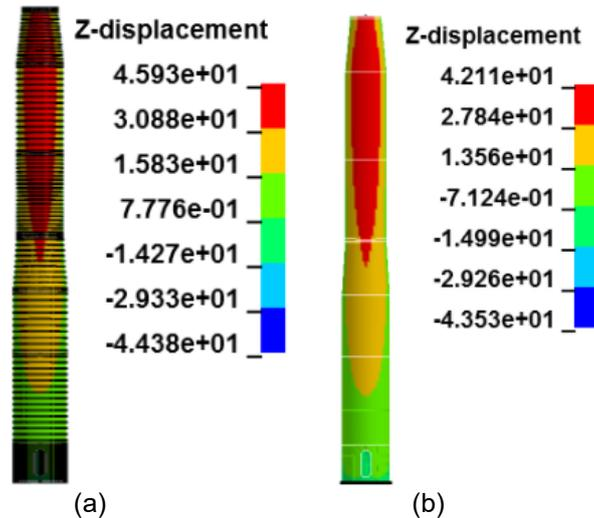
Fig. 17: The first vibration mode (a) IGA; (b) FEA.
