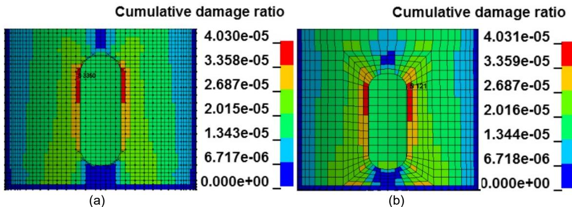
Fig. 20: The cumulative damage ratio (a) IGA; (b) FEA.
