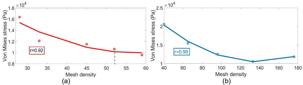
Fig. 10: Convergence results and the related correlation coefficient  $r$  of the fitting curves for (a) IGA (b) FEA.
