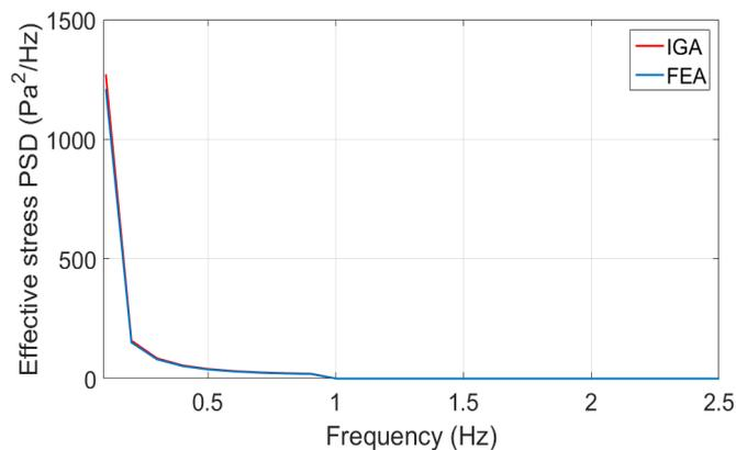
Fig. 18: The effective stress PSD.
