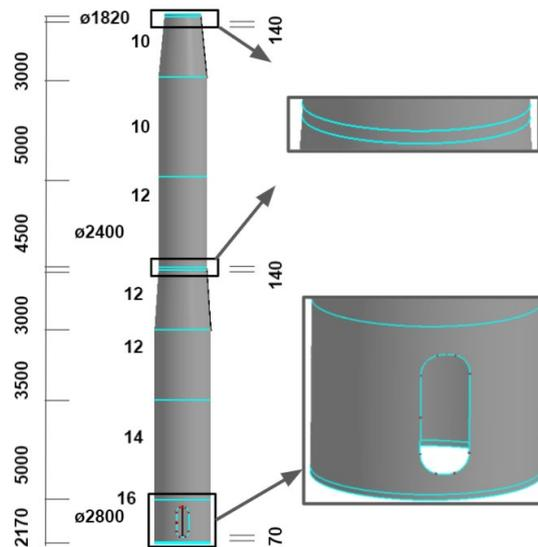
Fig. 15: Geometry model of the tower.
