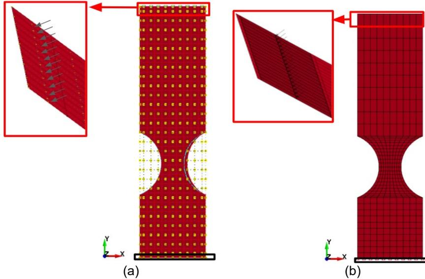
Fig. 9: Mesh models and boundary conditions (a) IGA; (b) FEA
