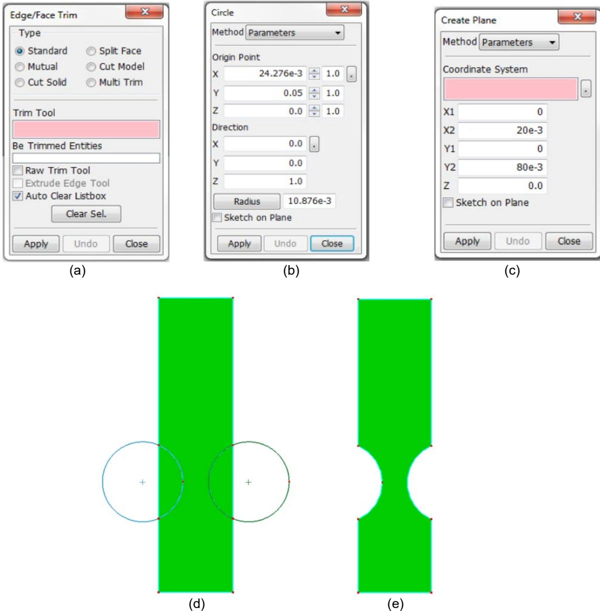
Fig.1: The geometry construction (a) Plate construction; (b) Circle construction; (c) Geometry trimming; (d) Created model; (e) Final mode).
