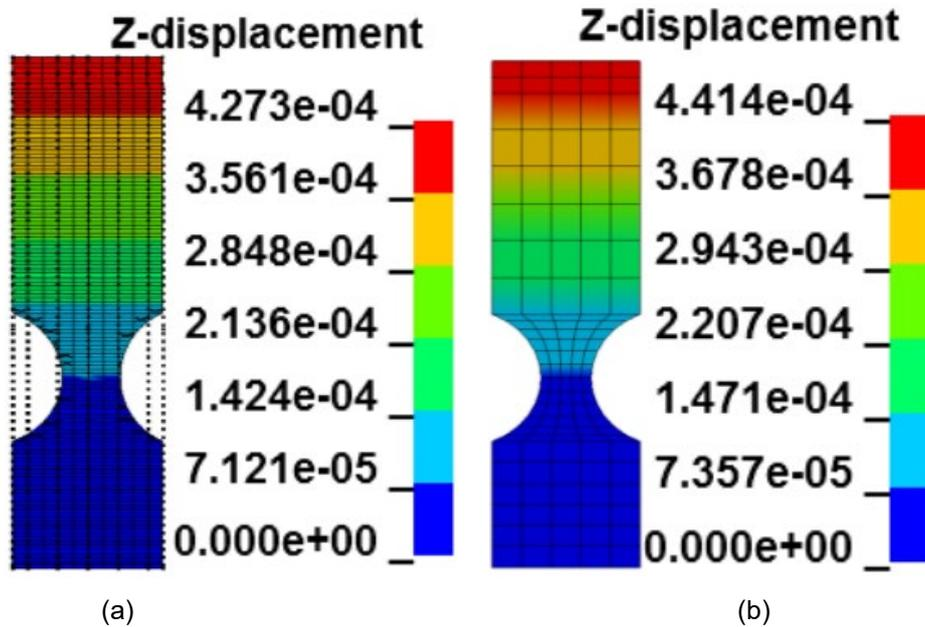
Fig. 11: The first vibration mode (a) IGA; (b) FEA.
