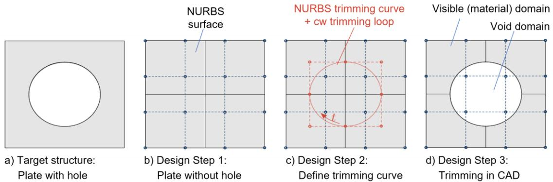
Fig.3: The logic of a trimming operation in CAD
