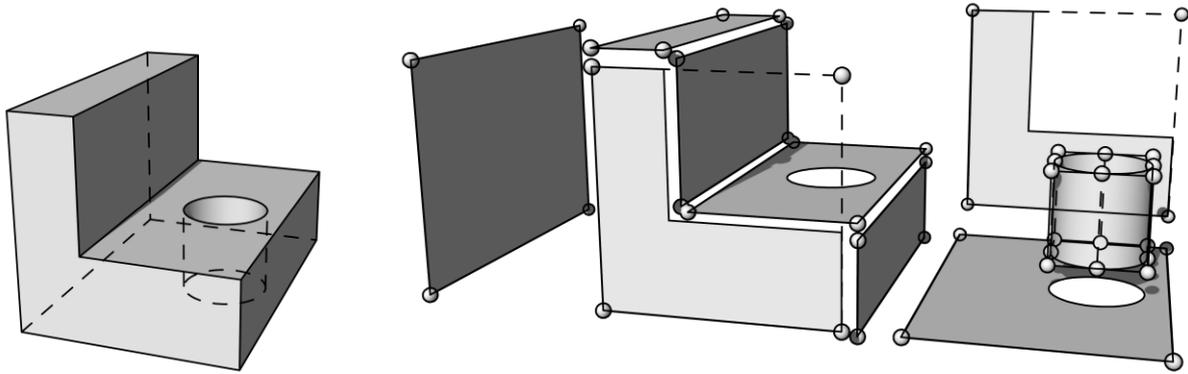
Fig.1: 3D object (left) and NURBS-based B-Rep model (right) [2]
