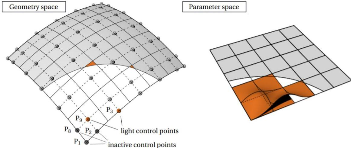
Fig.6: Small trimmed elements with light control points (left) and the corresponding NURBS basis functions (right) [7]
