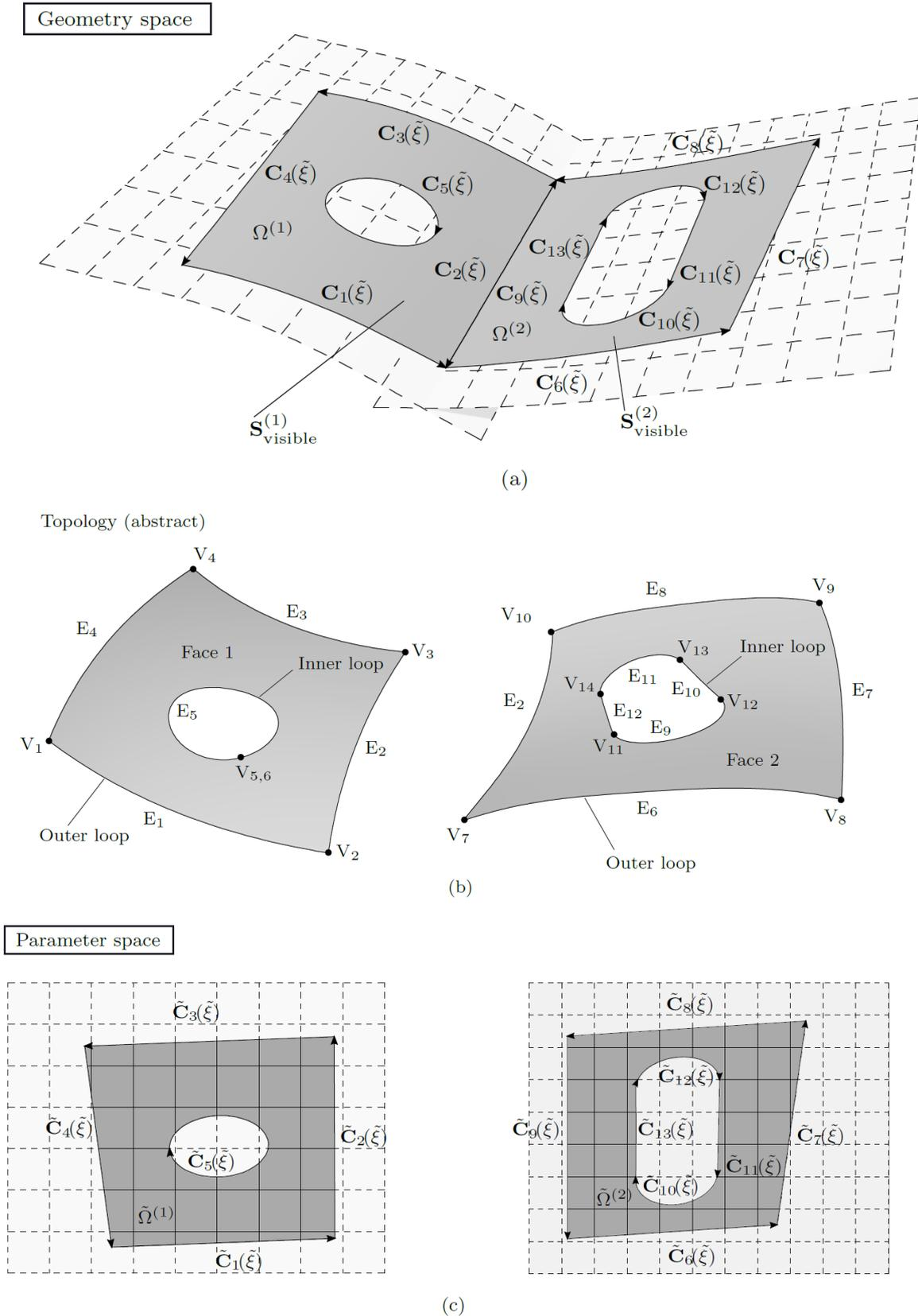
Fig.4: Trimmed surface B-Rep model represented in geometry space, as abstract topology and in parameter space, taken from Leidinger et al. [3]
