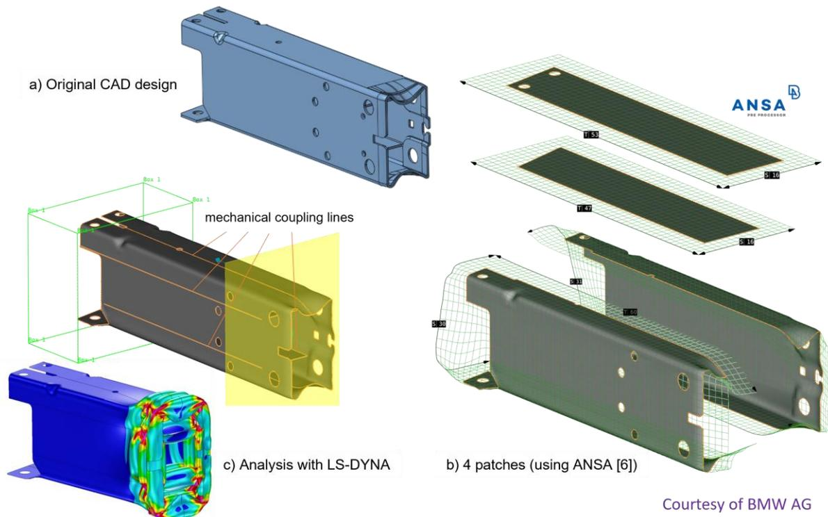
Fig.5: Crashbox model: From CAD design to LS-DYNA analysis
