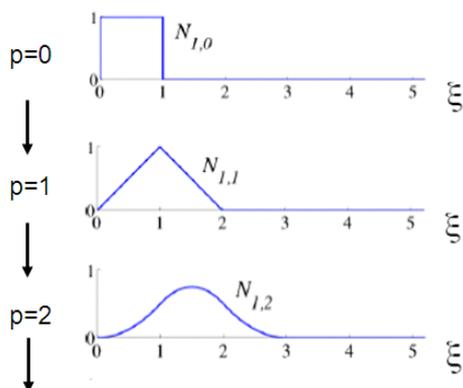
Fig.2: B-spline basis functions of order 0,1 and 2 for uniform knot vector [1]
