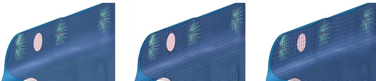
Fig.7: Spotwelds between IGA shells modeled via `*CONSTRAINED_INTERPOLATION_SPOTWELD` with visualized interpolation elements of sheet 1 (middle) and sheet 2 (right)
