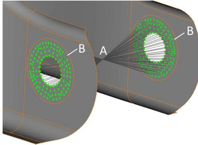
Fig.8: A `*CONSTRAINED_NODAL_RIGID_BODY` attached to IGA shells via `*IGA_POINT_UVW` (highlighted in green)
