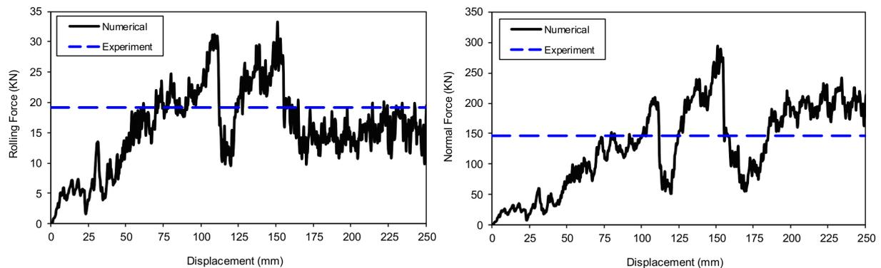
Fig.6: Rolling and normal force applied to the disc cutter
