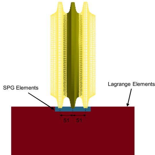
Fig.11: Finite element model (spacing: 51 mm)
