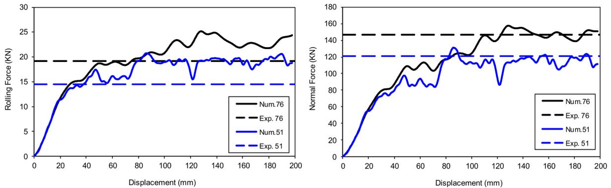
Fig.12: Effect of spacing distance on forces applied to the disc cutter
