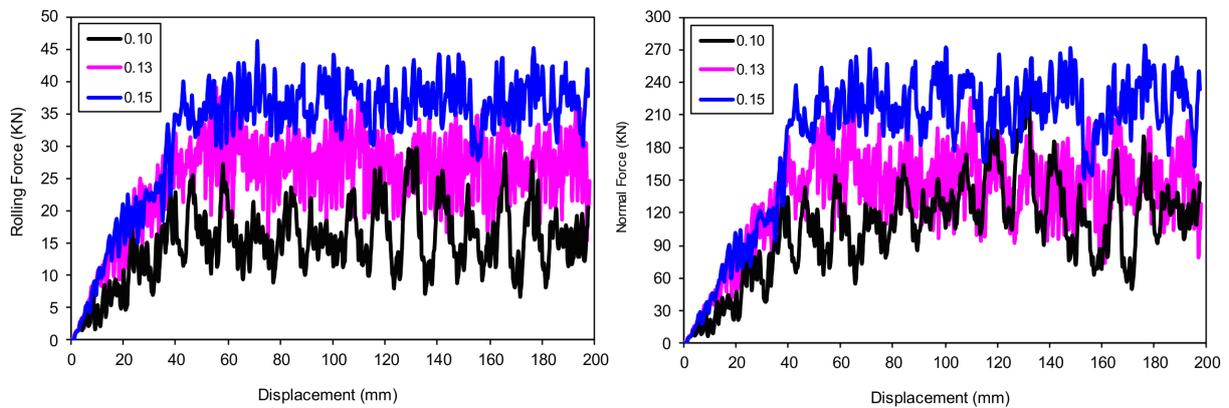
Fig.4: Effect of value of the MXEPS on forces applied to the disc cutter
