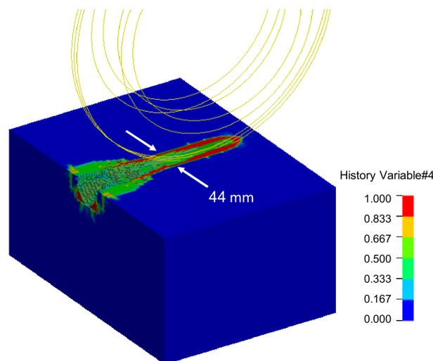
Fig.7: Damage created in the rock due to the movement of the disk cutter (RHT model)
