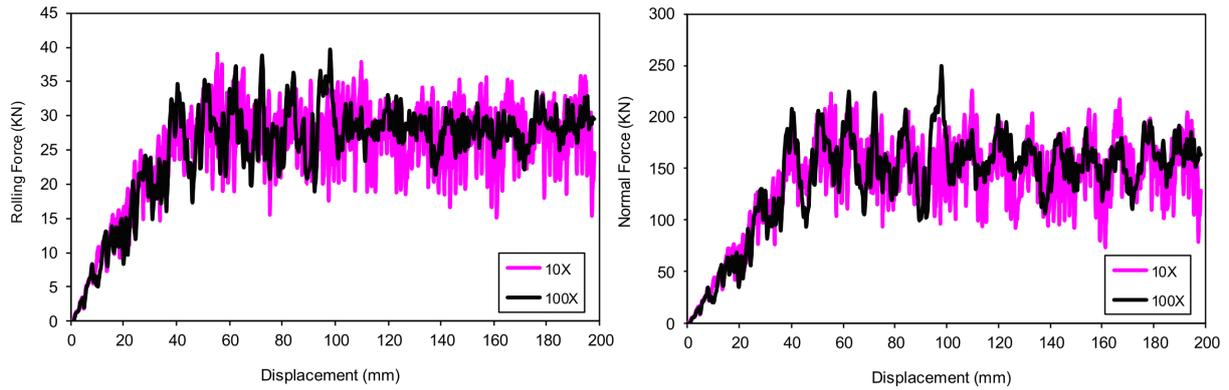
Fig.3: Effect of cutter velocity factor on forces applied to the disc cutter
