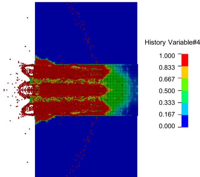
Fig.13: Damage caused to the rock by the movement of the cutter disc (spacing: 51 mm)
