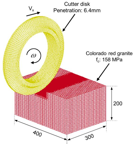
Fig. 2: Finite element model (dimensions are in millimeters)
