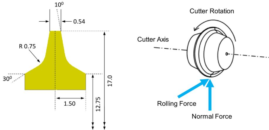
Fig. 1: Left: Dimensions of the cutter disc cross section (in inches), right: The forces applied to the disk cutter
