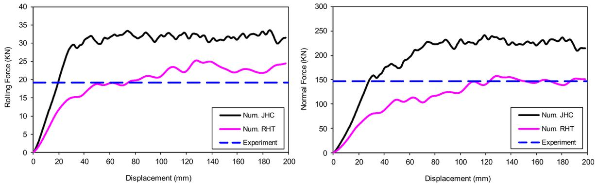
Fig.9: Rolling and normal force applied to the disc cutter
