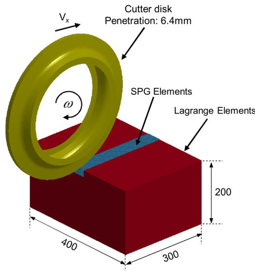
Fig.8: Finite element model (dimensions are in millimeters)
