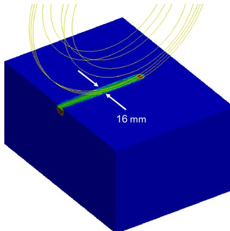
Fig.5: Damage created in the rock due to the movement of the disk cutter (JHC model)
