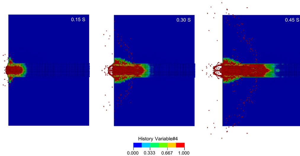
Fig.10: Damage created in the rock due to the movement of the disk cutter
