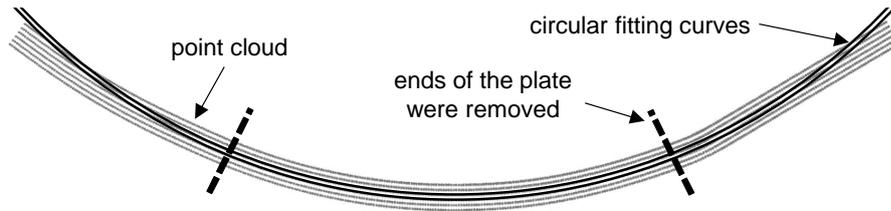
Fig.6: Determination of the radius of a plate after rolling simulation.
