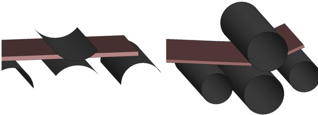
Fig.3: Modelling of the rolls by rigid shells in the bending step (left) and contact entities in the rolling step (right).
