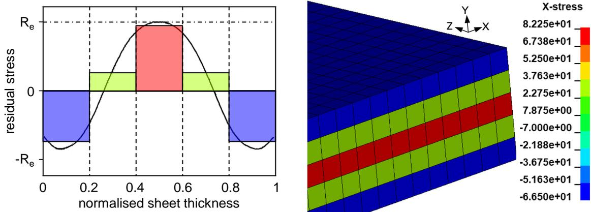
Fig.5: Left: Adaptation of the residual stress curve from [13] for implementation in the model. Right: Section of the FE model of a plate with implemented residual X-stresses (S355, scaling factor of the residual stress state = 0.25).
