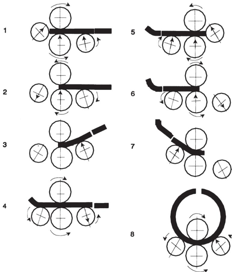
Fig.2: Operational sequence for thick plate bending process with a 4-roll plate bending machine [10].
