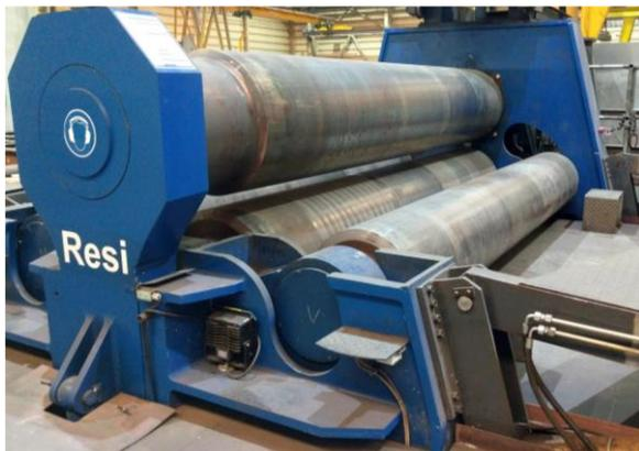
Fig. 1: Modelled 4-roll plate bending machine.
