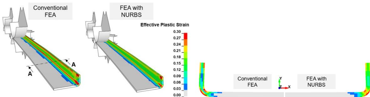
Fig. 11: Comparison of effective plastic strain overview (left) and section (right) at the third and last stand
