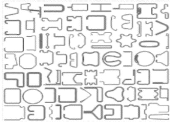
Fig.2: Some examples of roll formed profiles, courtesy of UBECO GmbH
