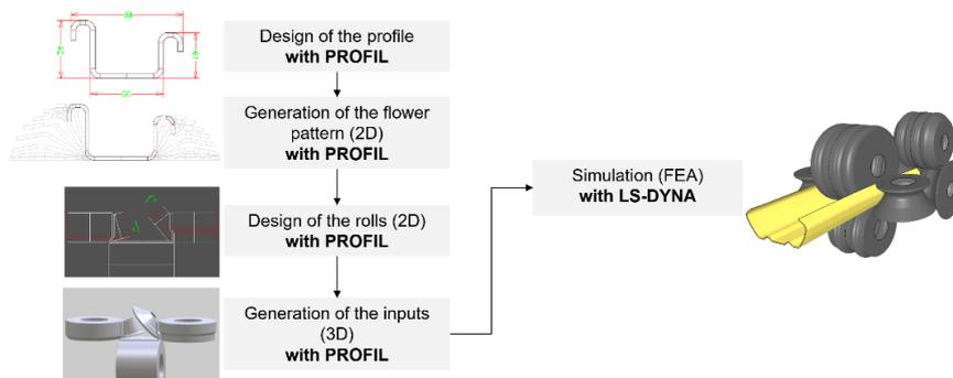
Fig.6: Overview how to create the simulation inputs from the final profile cross section
