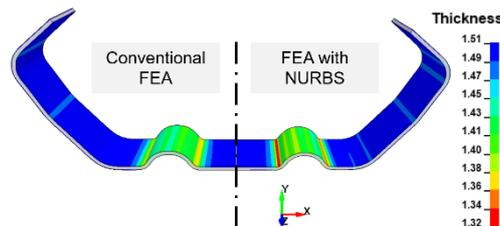
Fig. 16: Comparison of thickness reduction after the last stand for a small portion of the strip
