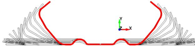
Fig. 13: Flower pattern of the bumper-profile. The final profile section is represented in red
