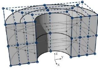
Fig.5: NURBS solid with the control points (blue dots) in physical space [4]
