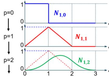
Fig.4: B-spline basis functions of order 0, 1 and 2 for uniform knot vector [2]
