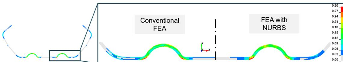
Fig. 15: Comparison of the effective plastic strain section at the last stand
