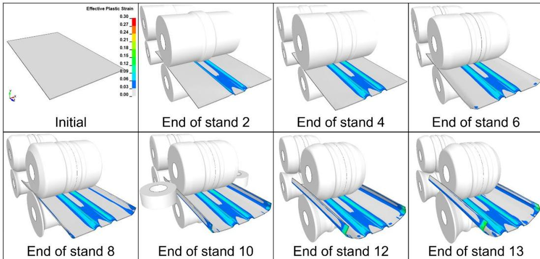
Fig. 14: Overview of the effective plastic strain at the end of some stands for IGA model
