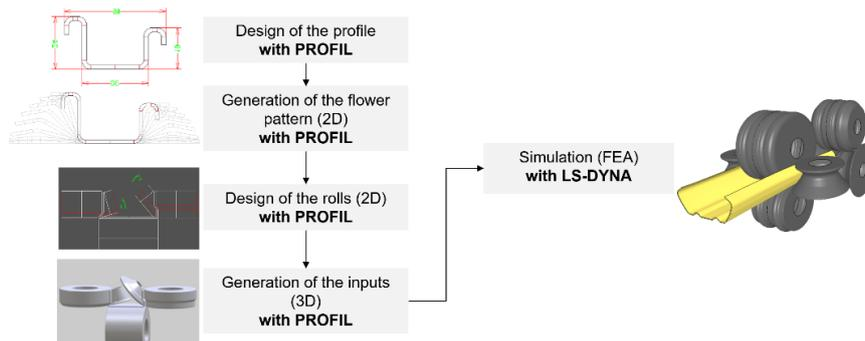
Fig.6: Overview how to create the simulation inputs from the final profile cross section
