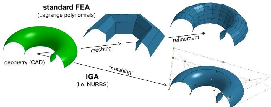
Fig.3: Comparison of meshing for standard finite elements and IGA
