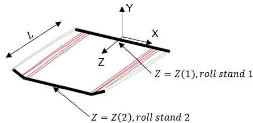
Fig.8: Example of a deformed sheet between roll stand 1 and 2
