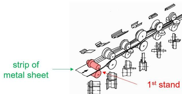
Fig. 1: Principle of the roll forming process, courtesy of UBECO GmbH
