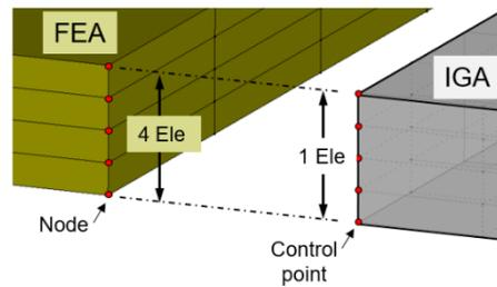
Fig.9: Finite element meshing and NURBS-solid for the strip
