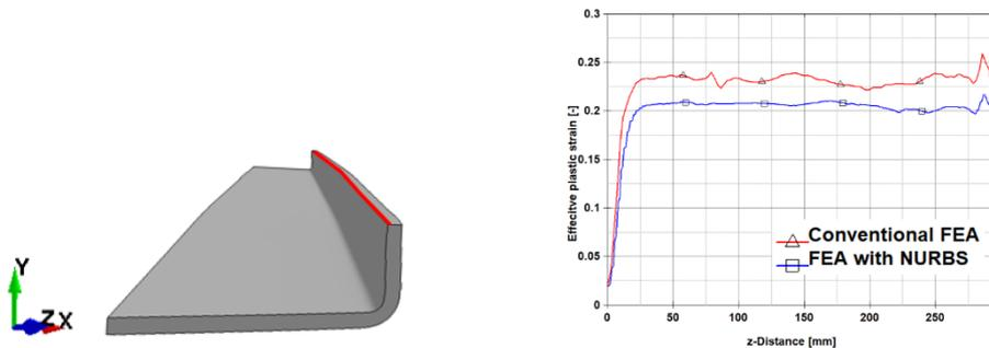
Fig. 12: Comparison of effective plastic deformation in function of the Z-distance (right) along the edge (left) at the third and last stand
