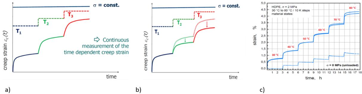
Fig. 6: Illustration of the Stepped Isothermal Method; a) Measurement of the creep strain; b) Subtracting thermal strains; c) Example of resulting creep curves [7]
