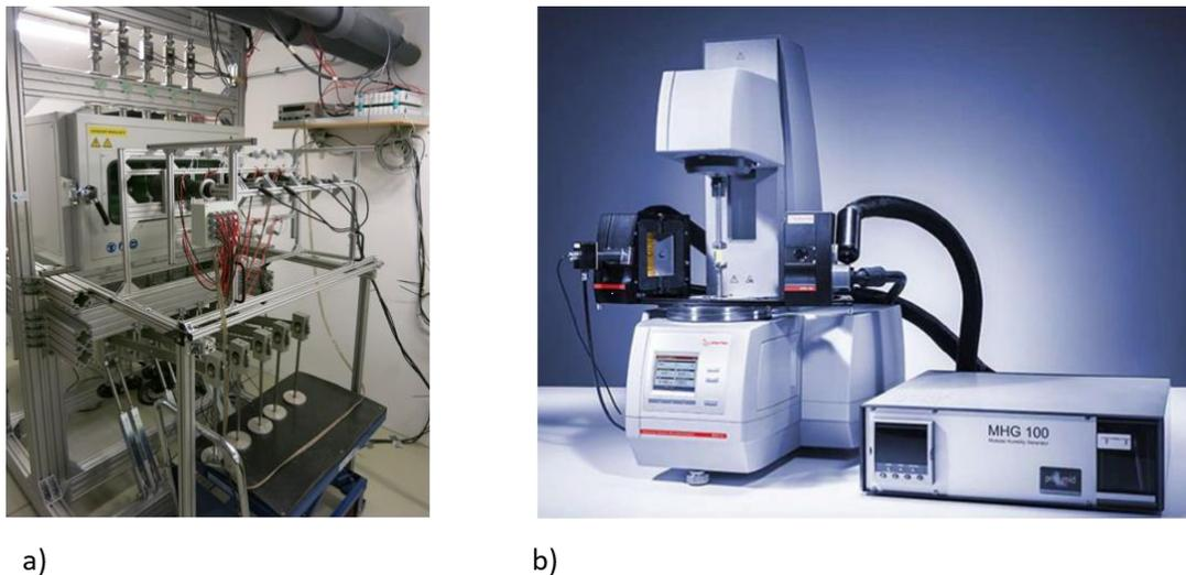
Fig. 5: Devices for creep testing; a) Self constructed 5-fold creep test rig; b) Anton Paar DMA MCR 702e MultiDrive
