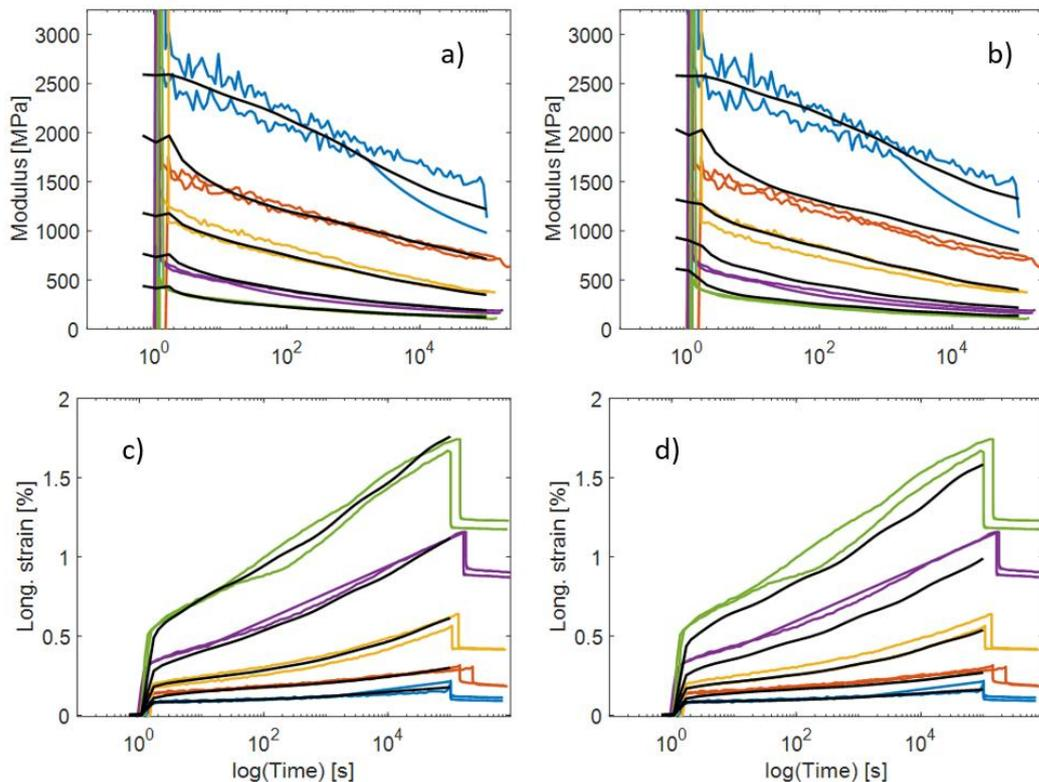
Fig. 11: Verification results on specimen level; a) \*MAT\_076 prediction of the creep modulus; b) \*MAT\_002+MAI prediction of the creep modulus; c) \*MAT\_076 prediction of the strain behavior ; d) \*MAT\_002+MAI prediction of the strain behavior
