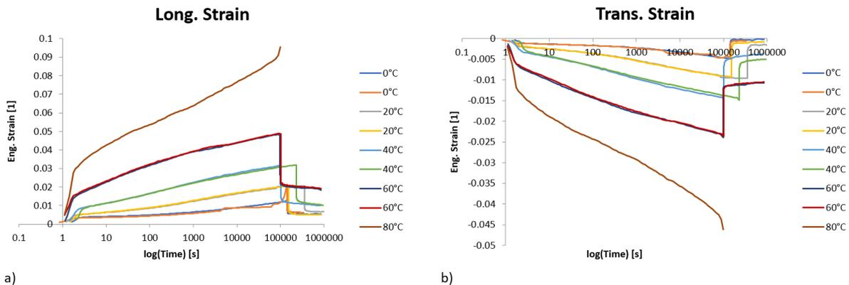
Fig. 7: a) Creep behavior at 5 MPa load of PE in longitudinal direction; b) Creep behavior at 5 MPa load of PE in transverse direction.
