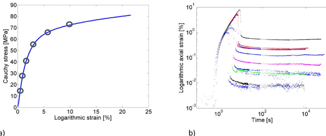
Fig. 3: Strain-Recovery Method; a) Schematic creep loads for strain-recovery measurements; b) Creep-recovery behavior
