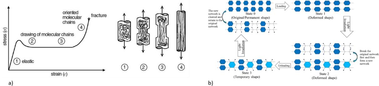
Fig. 12: Stress-strain behavior of thermoplastic polymers during tensile testing
