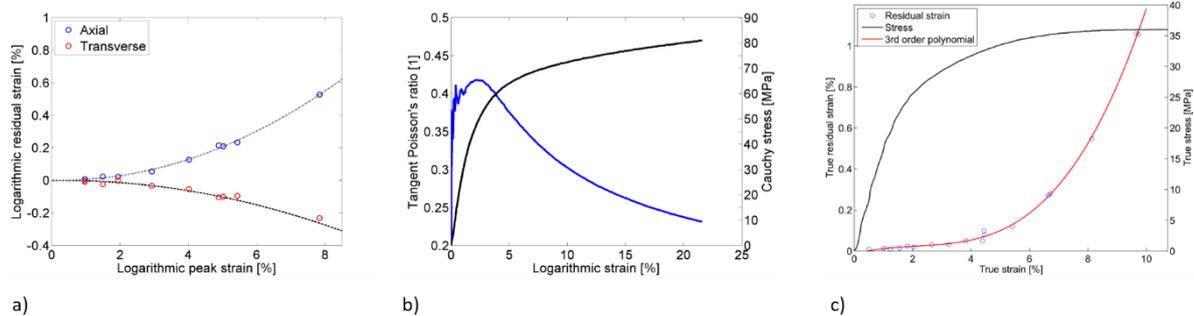
Fig. 4: Determination of irreversible strain; a) Evolution of residual strain with time; b) Tangent Poisson's ratio describing the total strain behavior; c) Residual strains after recovery
