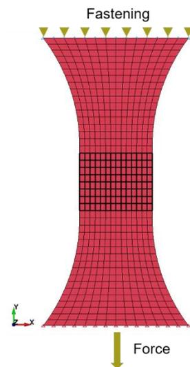
Fig. 9: Simulation model
