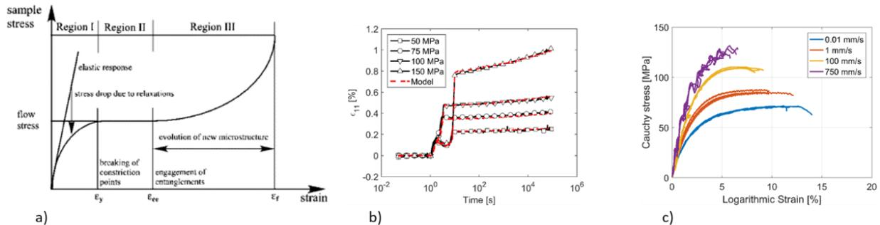
Fig. 2: Mechanical response of thermoplastics; a) Schematic overview with regard to the stress-strain behavior [2]; b) Creep behavior at different load levels [3, 4]; c) Strain rate dependency [5]
