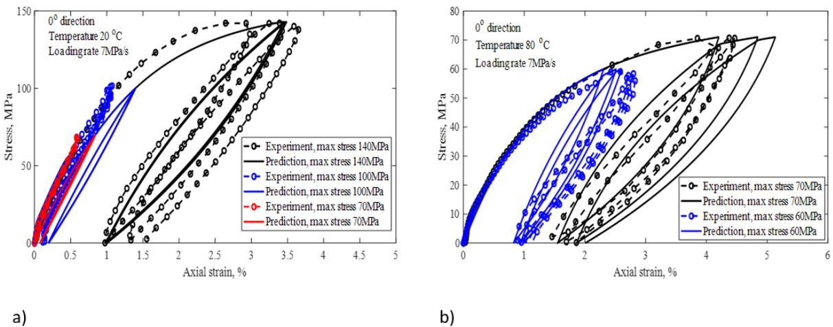
Fig. 15: Loading-Unloading behavior at a) room temperature and b) 80°C using the nonlinear model approach
