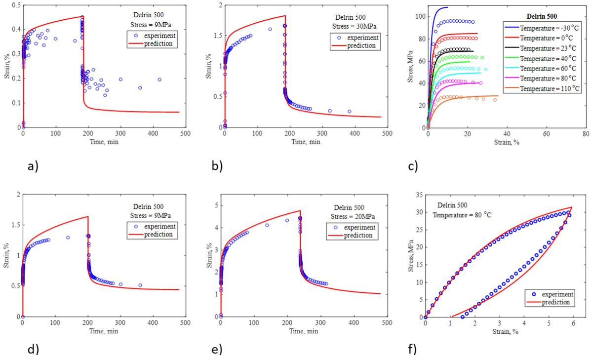
Fig. 14: Validation simulation nonlinear model; a) Creep-recovery at 23°C and 9MPa; b) Creep-recovery at 23°C and 30MPa; c) Creep-recovery at 80°C and 9MPa; Creep-recovery at 80°C and 20MPa; e) Tension; f) Loading-Unloading [10]
