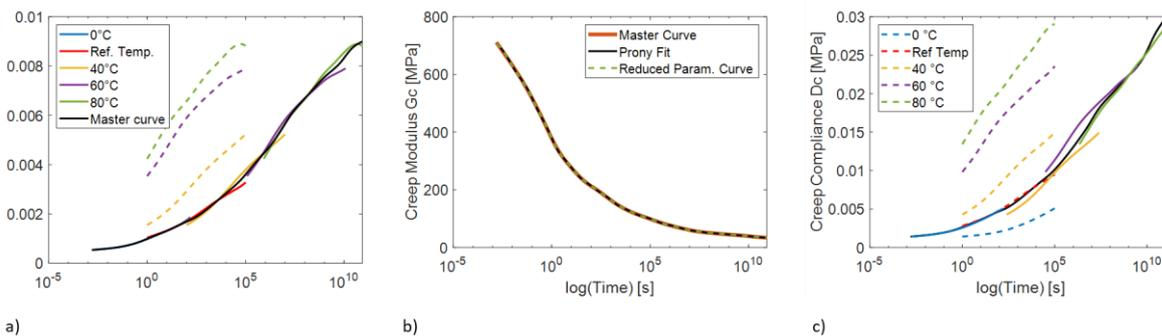
Fig. 8: Determination of model parameters; a) Generation of a master curve; b) Prony-parameter optimization using e.g. nonlinear least squares method; c) WLF-parameter optimization using e.g. nonlinear least squares method
