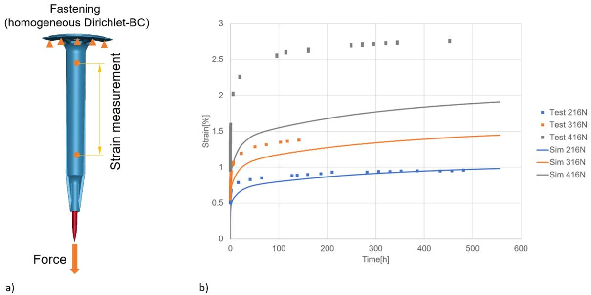
Fig. 10: Validation model and results on component level; a) Simulation model of an insulation board anchor; b) Simulation results using a linear viscoelastic model corresponding to 216N loading
