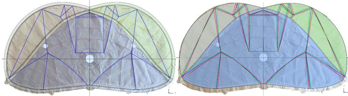
Fig.4: Left: PAB with hem, foldline beams in blue. Right: Simple no-hem model, three foldline patterns in red, green and blue superimposed
