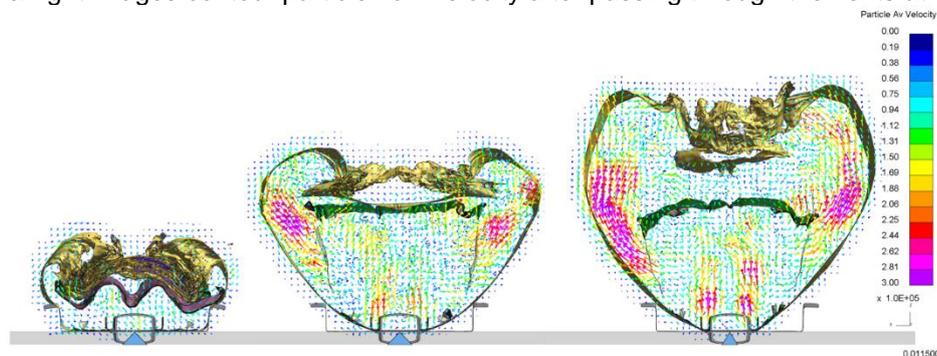
Fig. 18: Averaged/smoothed particle flow velocity at 6ms, 8.5ms & 11.5ms, visualized in Oasys D3PLOT
