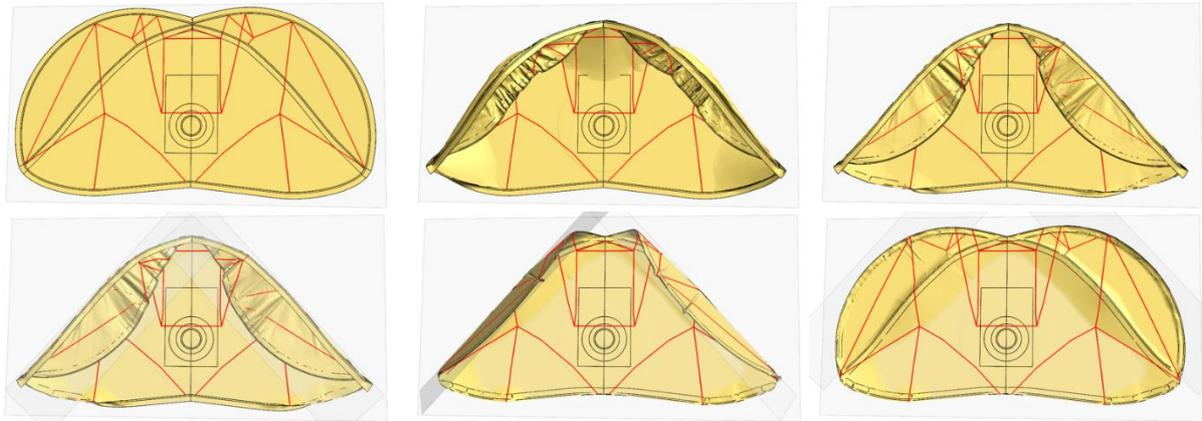
Fig.6: Turning the pre-stitched side panels inside out so that the hem lies on the inside
