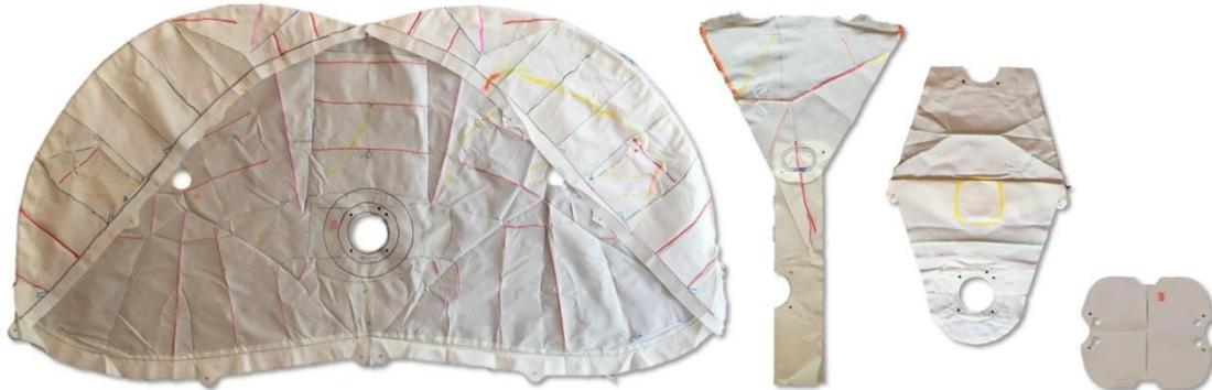
Fig.2: Left: main panel semi-assembled, hem tucked inside, foldlines marked in pen. Right: tether, inner & wrapper.
