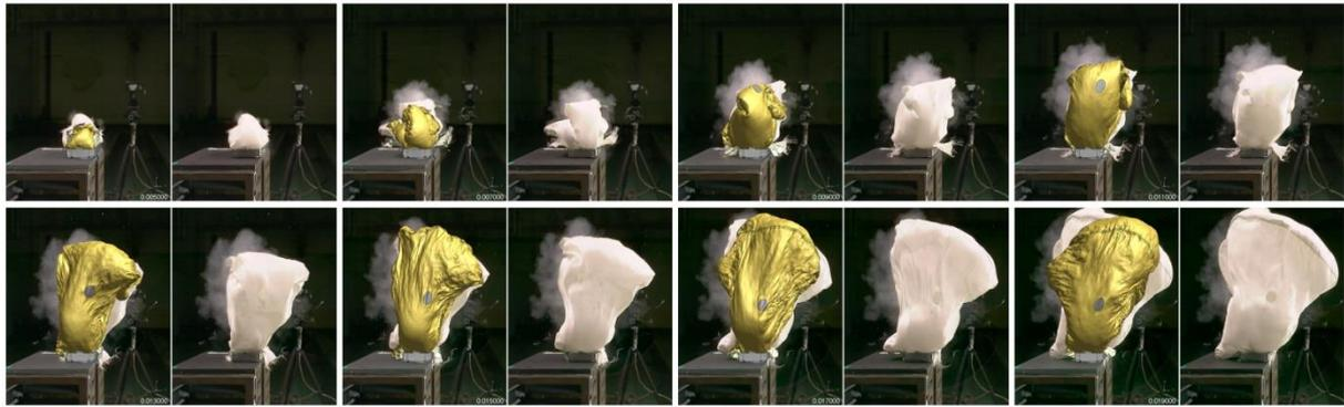
Fig. 16: Static deployment vs test, view from side (2ms between frames)
