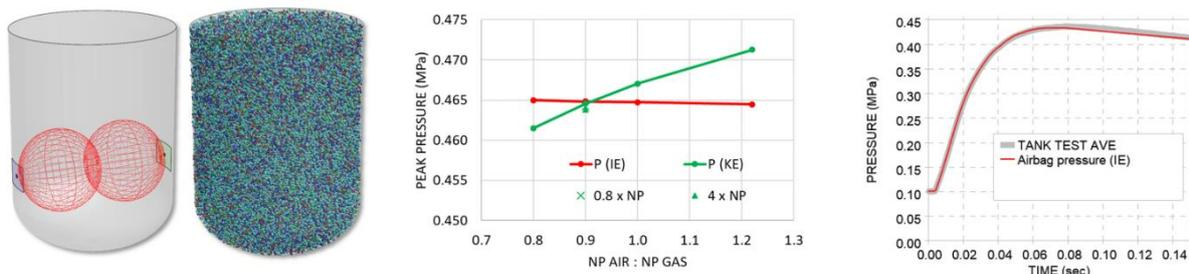
Fig.15: Left: tank test model with CPM sensors. Middle: differences in peak pressure reported by "Airbag pressure" P (IE), and "Particle pressure" P (KE) for varying ratios of NP air:gas. Right: tank test vs. analysis pressure P(IE)
