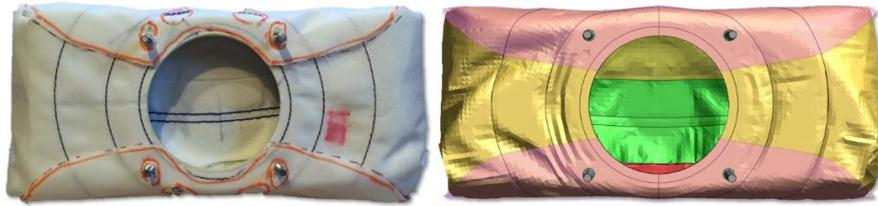
Fig.10: Folded & fitted with retainer & wrapper, view from below.
