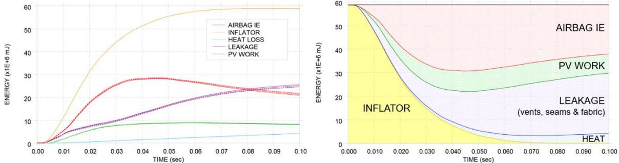
Fig.20: Airbag energies without dummy. Left: all cases, right: energy flow in a typical case
