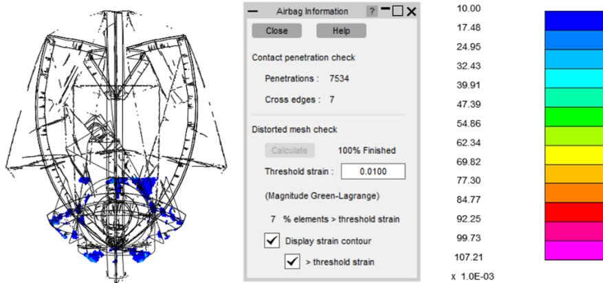
Fig.14: JFOLD's quality checks include number of crossed edges and residual strain
