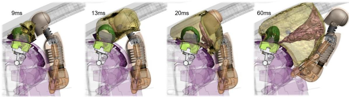
Fig.22: Key events during Position 1 deployment
