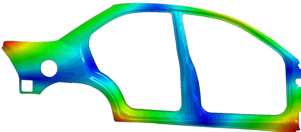
Fig.8: The seventh mode (first non-rigid body mode) of an isogeometric, boundary-fit shell of the outer-right portion of the chassis of a 1996 Dodge Neon defined using cubic NURBS patches is shown.
