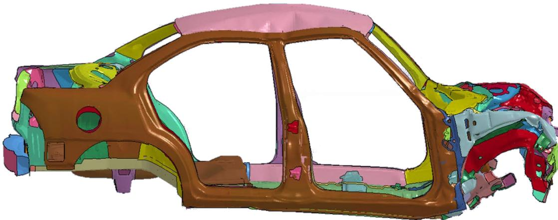
Fig.11: After replacing the outer-right shell of the vehicle chassis (in brown, replacing the orange shell of Fig. 9, and shown in Fig. 8) with an isogeometric bicubic shell, the chassis of the 1996 Dodge Neon crash model from [15] is shown after frontal crash loading. This model uses a single isogeometric component, with all others being the mesh elements from [15].
