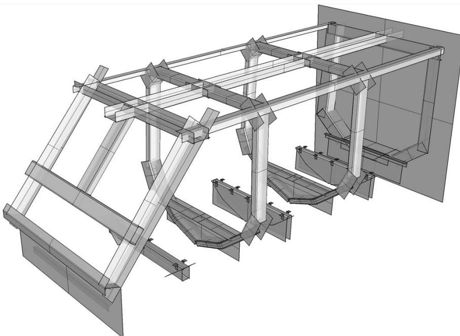
Fig.2: The untrimmed structural components of the DEVCOM Generic Hull vehicle are shown.
