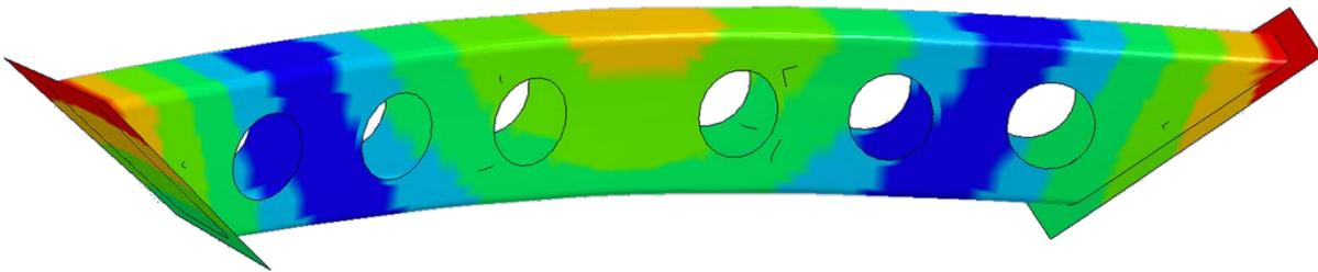
Fig.7: The seventh mode (first non-rigid body mode) of an isogeometric, boundary-fit beam assembly in the DEVCOM Generic Hull is shown, defined using cubic NURBS patches.
