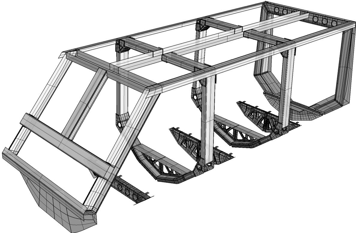
Fig.5: Rebuilt smooth Beziér patches the US Army's DEVCOM Generic Hull vehicle constructed using the proposed method are shown. Splines were computed using the trimmed CAD geometry of Fig. 1 as input.
