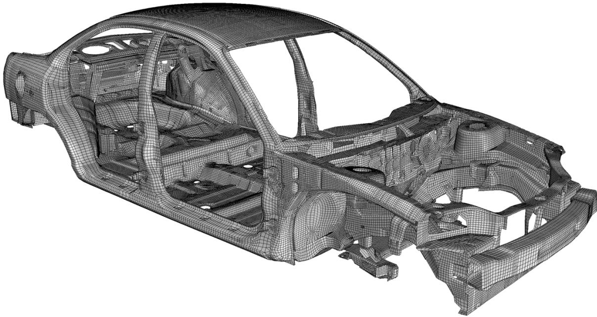
Fig.3: The NCAC's finite element mesh of a 1996 Dodge Neon chassis, from [15], is shown for reference. Compare this mesh to the reconstructed model shown in Fig. 6.
