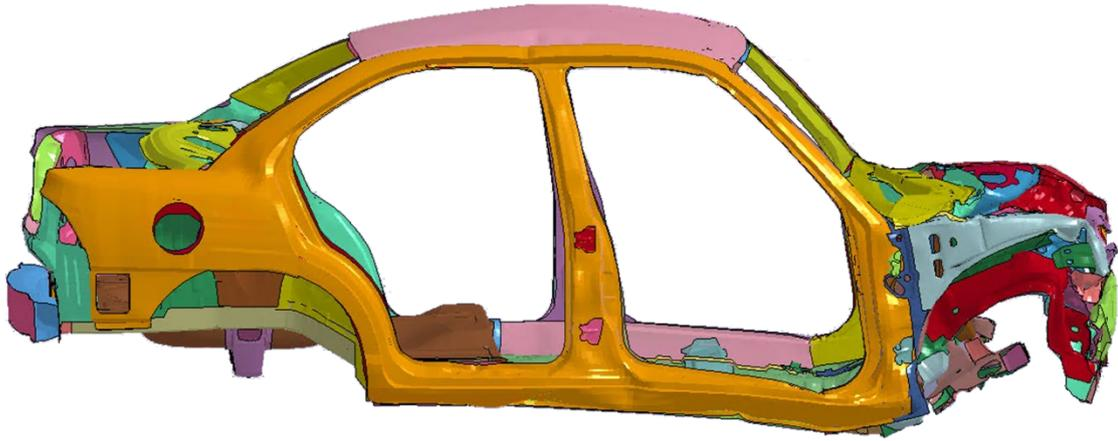
Fig.9: The chassis of the 1996 Dodge Neon crash model reproduced from [15] after frontal crash loading using traditional linear triangle and bilinear quadrilaterals elements is shown above.
