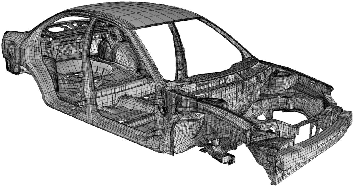
Fig.6: Rebuilt smooth B-spline surfaces of the NCAC's 1996 Dodge Neon constructed using the proposed method are shown. Splines were computed using the mesh of Fig. 3 as input.
