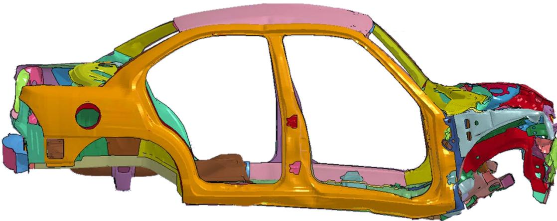
Fig.10: The chassis of the 1996 Dodge Neon crash model with outer-right shell (in orange) is refined to ~2mm resolution based on the original model of [15] and then subjected to frontal crash loading using traditional linear triangle and bilinear quadrilateral elements, as shown above.
