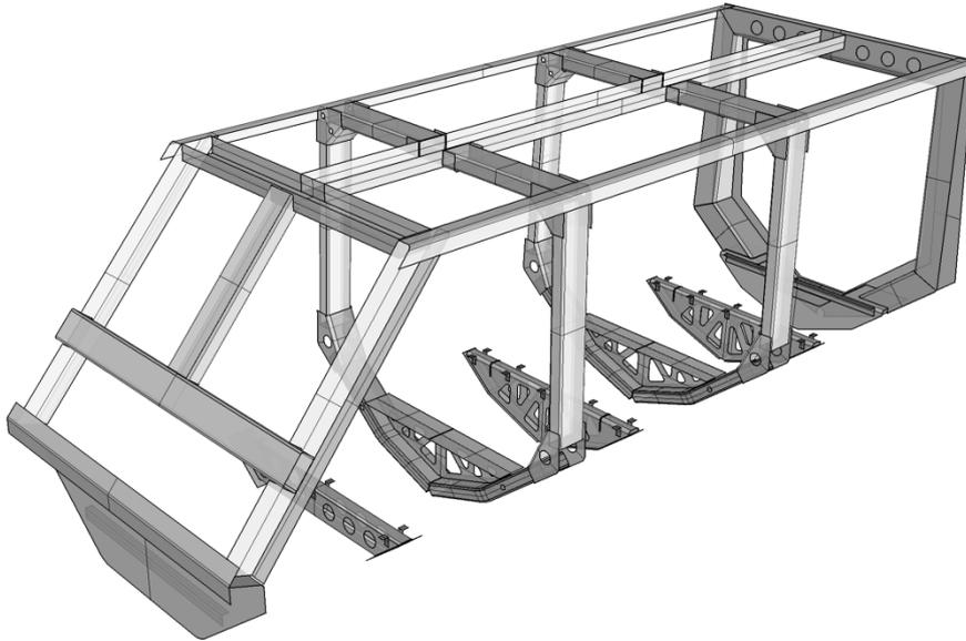
Fig.1: The trimmed structural components of the DEVCOM Generic Hull vehicle are shown. Compare this model to that of Fig. 5, after it has been reconstructed.
