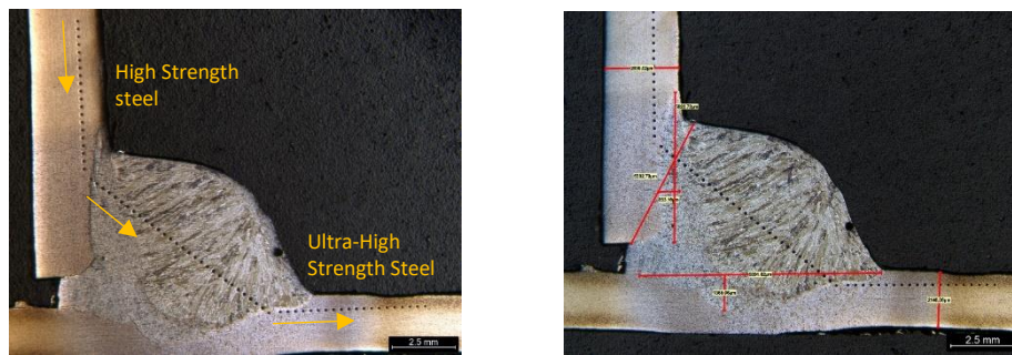
Fig. 6: Micro-Hardness Experiment at the weld joint area cross section
