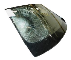
Fig.3: Fractured windshield after impact test 1 (other car parts are excluded from the image)
