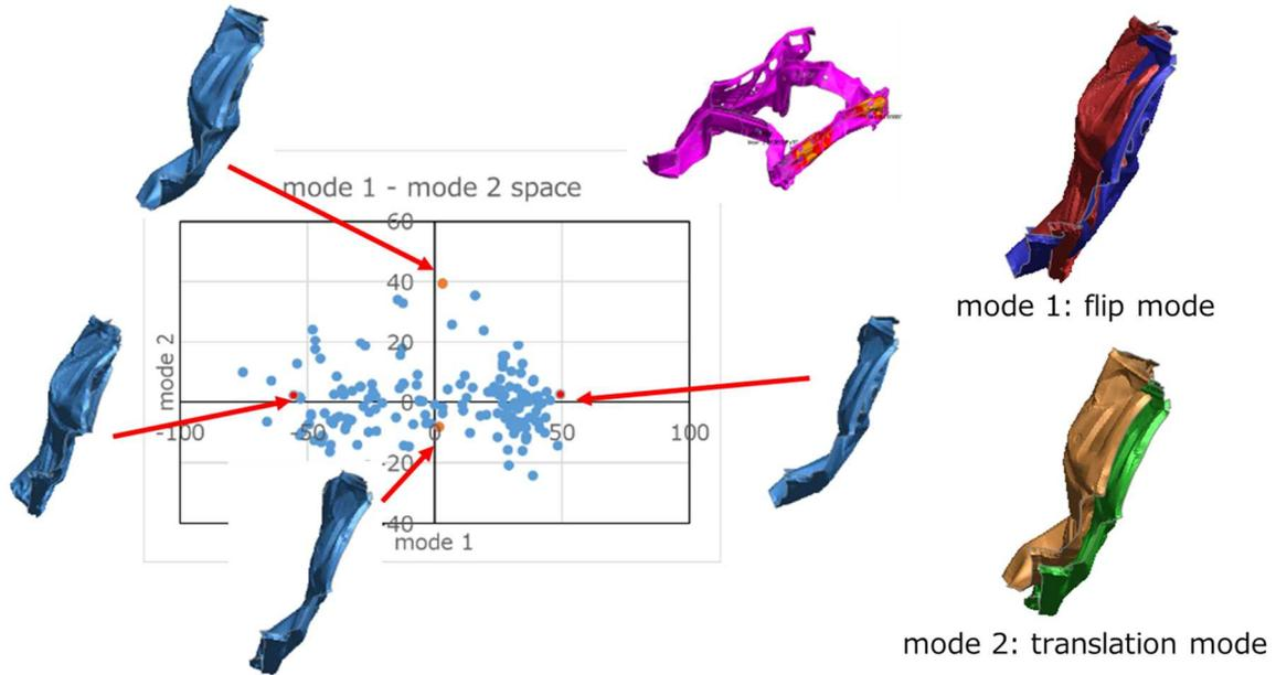
Fig.9: Modal plot with deformation mode of the firewall from the animation at 80ms
