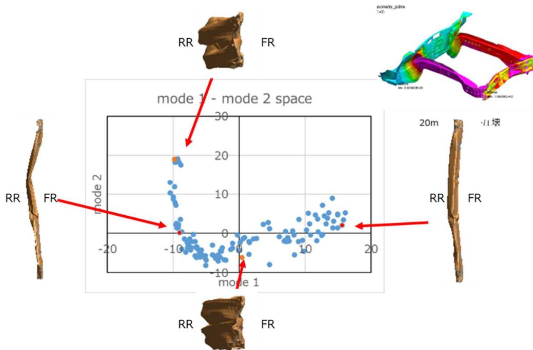
Fig.5: Modal plot with deformation mode of the bumper from the animation at 20ms
