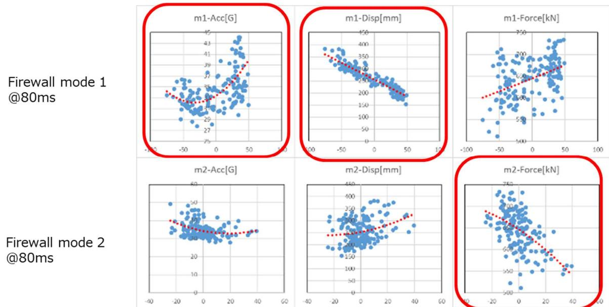
Fig. 16: Correlation between the modal contribution factors at 80ms and the output values
