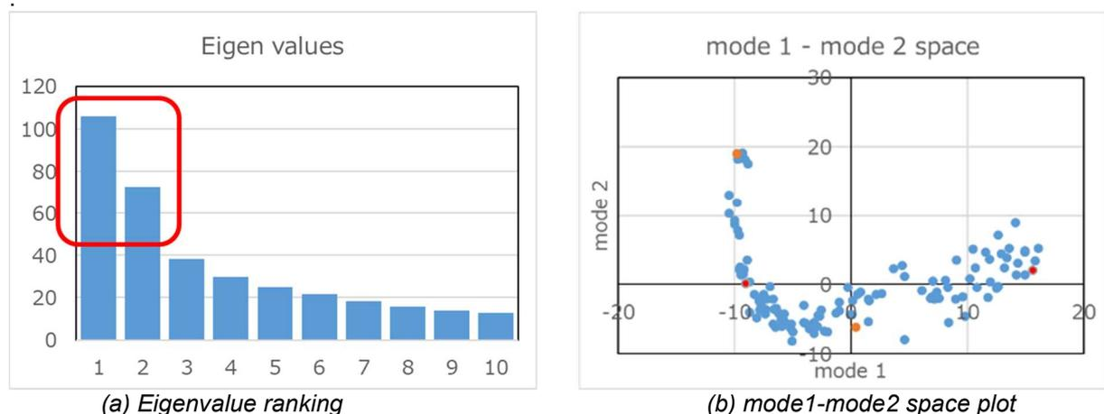
Fig.4: Result summary of PCA analysis of the bumper at 20ms
