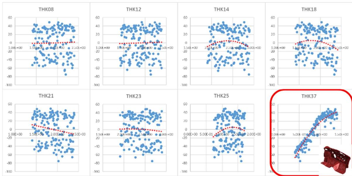
Fig.13: Correlation plot between the parameters and the first modal contribution factor at 80ms
