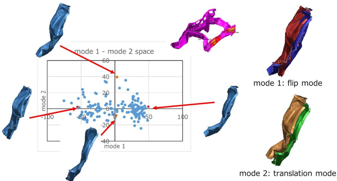
Fig.9: Modal plot with deformation mode of the firewall from the animation at 80ms
