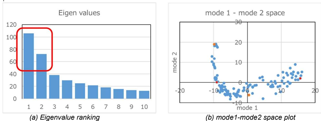
Fig.4: Result summary of PCA analysis of the bumper at 20ms
