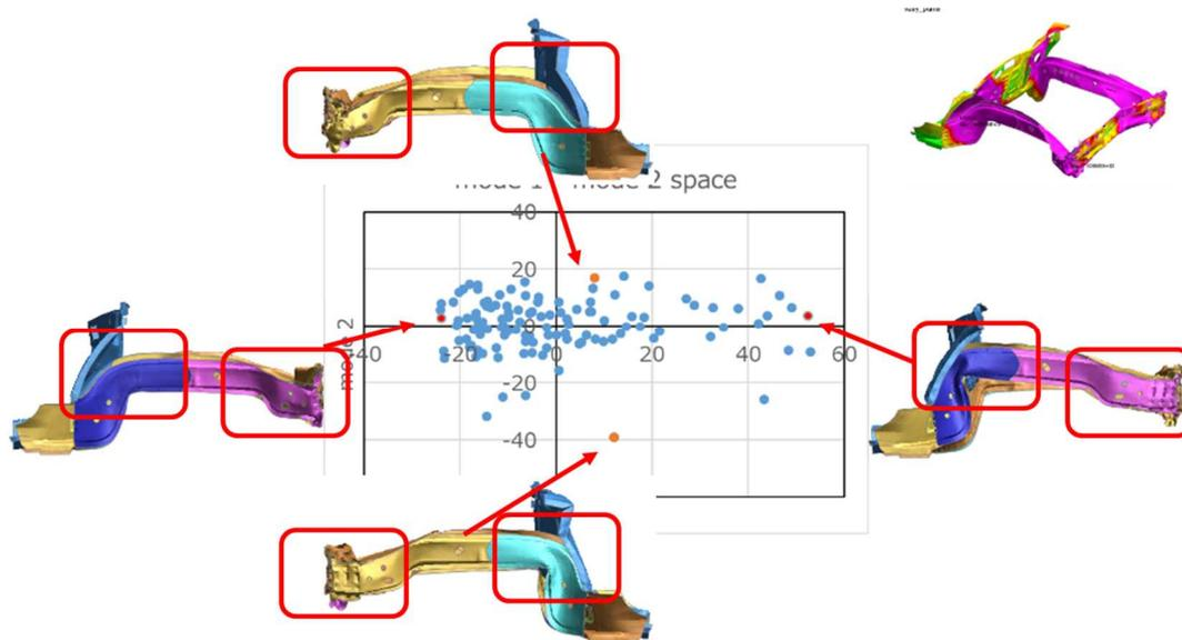
Fig.7: Modal plot with deformation mode of the front side members from the animation at 30ms
