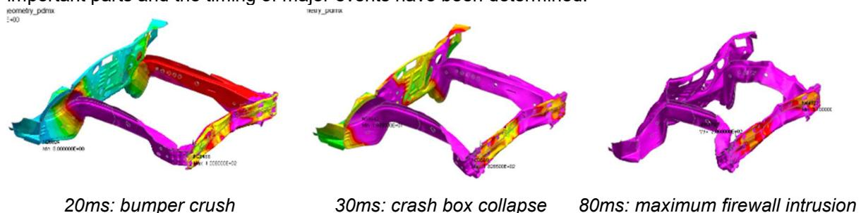
Fig.3: Scatter of important parts for the frontal crash.
