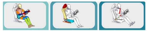
*Fig.14:* Calculating the dummy articulation, seat deformation and belt fastening process within the same simulation-driven positioning process with pre-defined processes.
