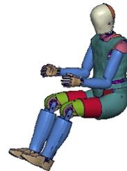
Fig.5: Used model for THOR 50% dummy
