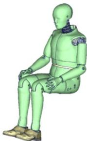
According to the test specification an ATD H350 must be seated at the passenger seat. In this case the virtual model from ATD-MODELS GmbH is used. This model was chosen for the project thanks to its handling easiness that couples perfectly with the GNS software solutions. On top of that, the model present enhancements such as:
