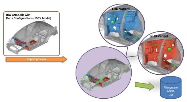
Fig.4: Multivariant Subsystem (BiW) with two Configurations (LHD and RHD).
