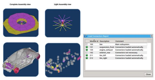
Fig.7: Assembly of Subsystems in full and lightweight view.
