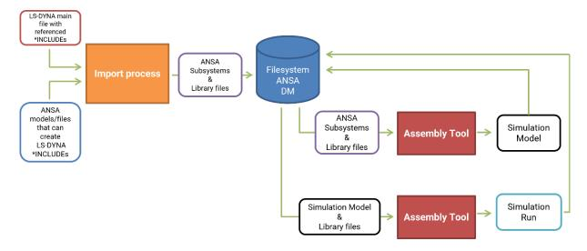
Fig.1: Workflow diagram.
