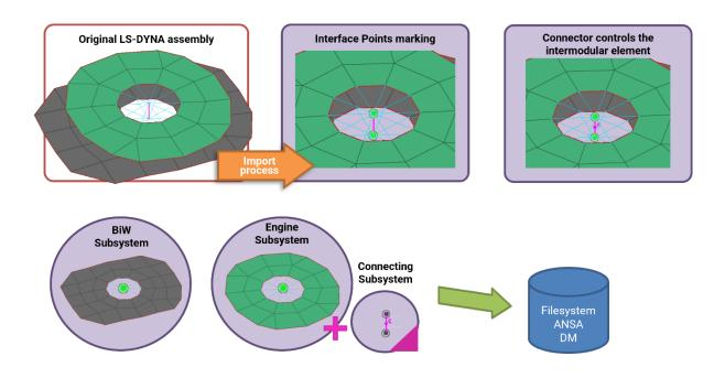
Fig.3: ANSA "A-Point - Connector - A-Point" concept for intermodular connection.
