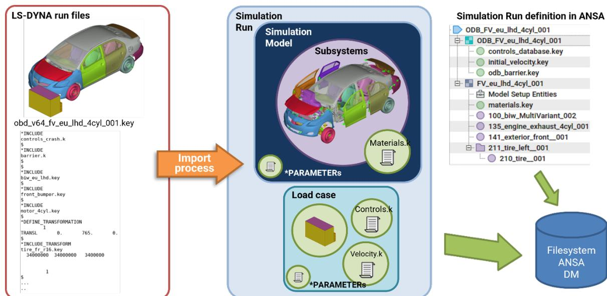
Fig.2: Import of an LS-DYNA run file into ANSA environment and ANSA DM.
