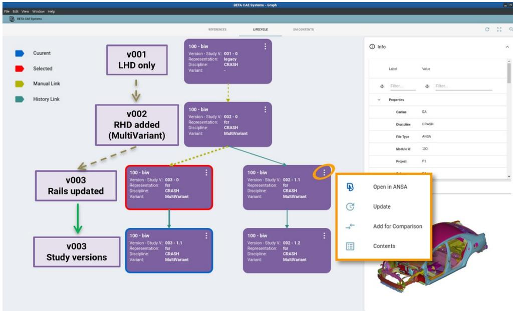
Fig.9: Lifecycle graph of an ANSA Subsystem.
