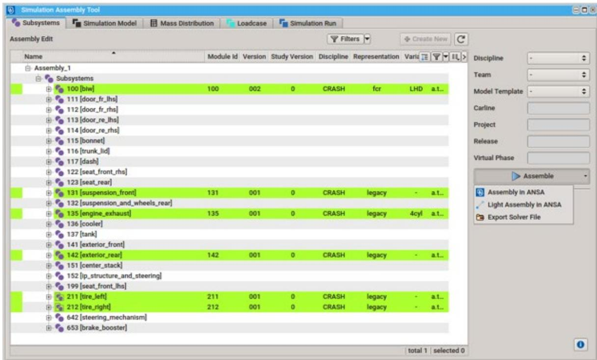
Fig.5: List of Subsystems available in ANSA DM.
