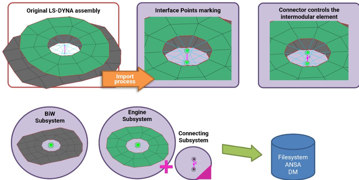
Fig.3: ANSA “A-Point – Connector – A-Point” concept for intermodular connection.
