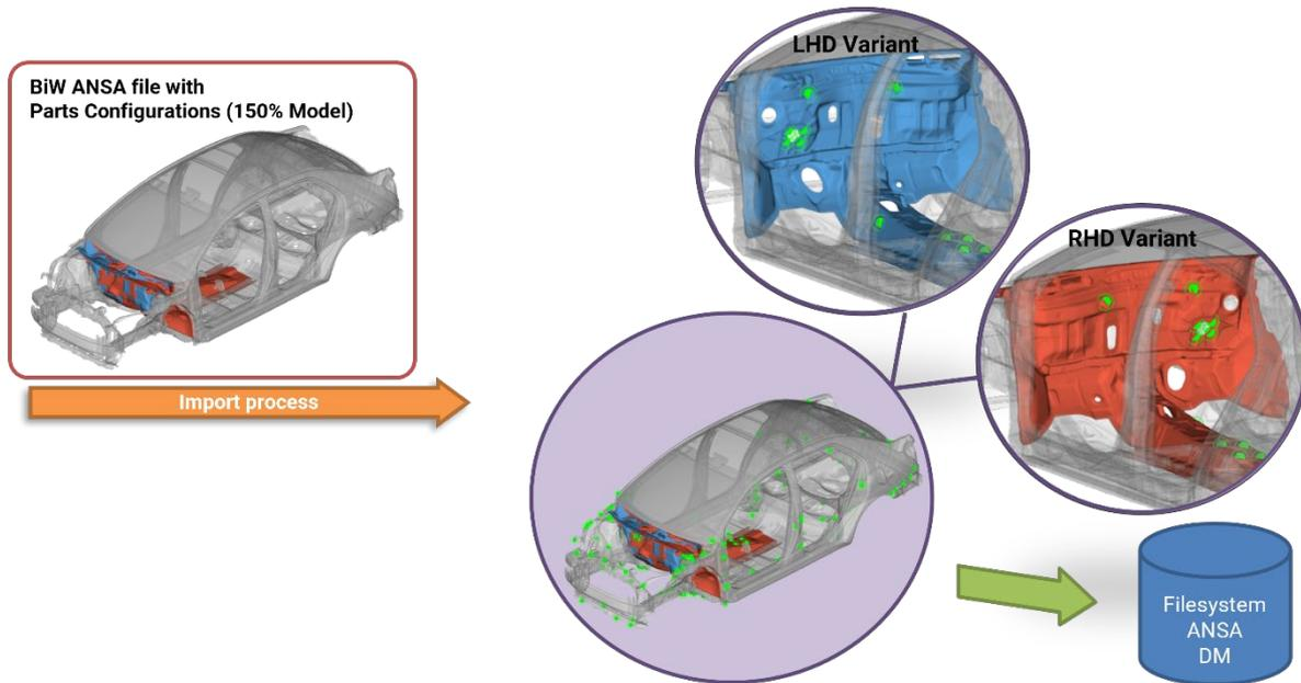
Fig.4: Multivariant Subsystem (BiW) with two Configurations (LHD and RHD).
