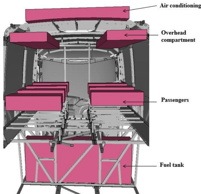
Figure 9 – Masses of non structural parts
