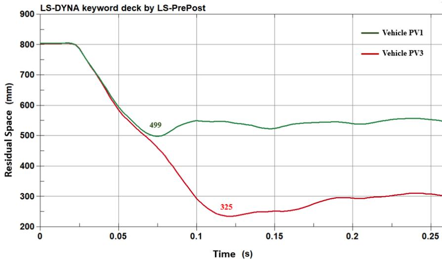
Figure 1 – Change in residual space after the collision for vehicle PV1 and PV3
