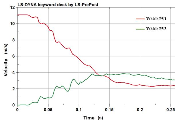
Figure 17 - Speed as a function of time
