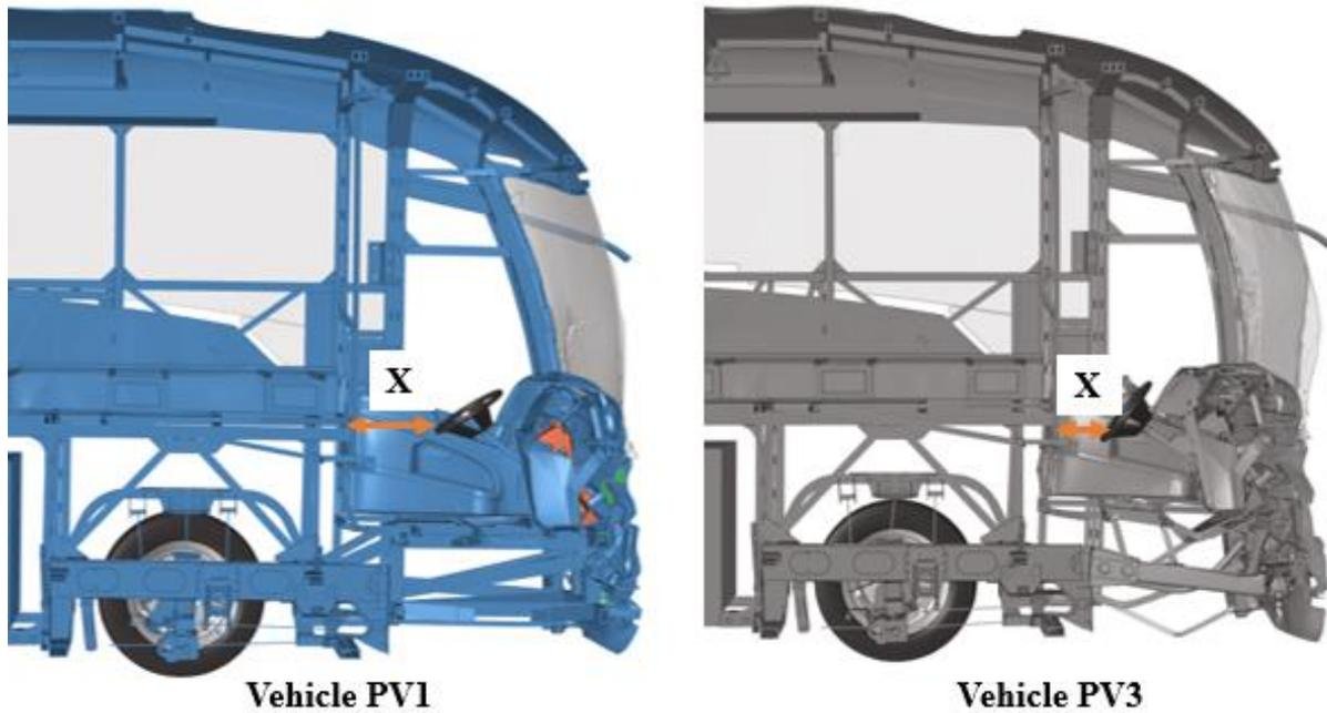
Figure 18 - Comparison of residual spaces
