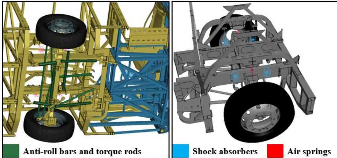
Figure 8 - Tension and stabilizer bars simplifications
