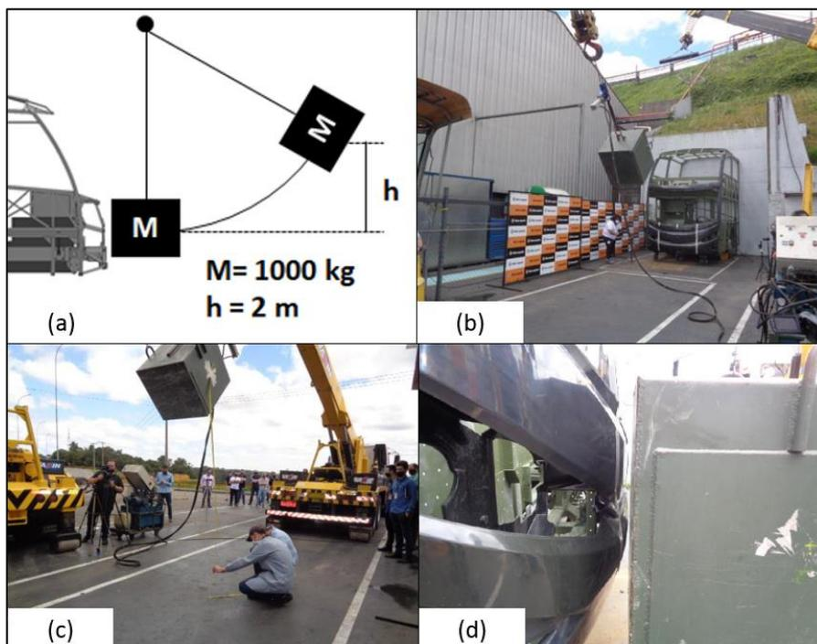
Figure 1 - Pendulum test according to CONTRAN Regulation No. 629
