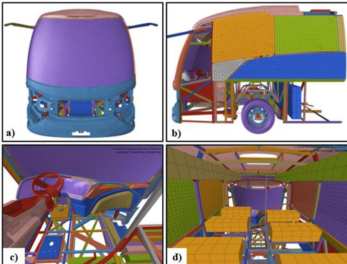
Figure 5 - Discretization of the numerical model
