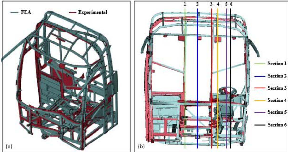
Figure 22 - Scanned model overlay and simulation
