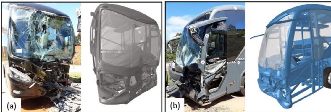
Figure 20 – Crash test (a) without FIA – (b) with FIA
