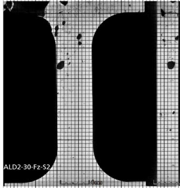
Fig.7: Two CT scan views of a tensile specimen with superimposed FE mesh.
