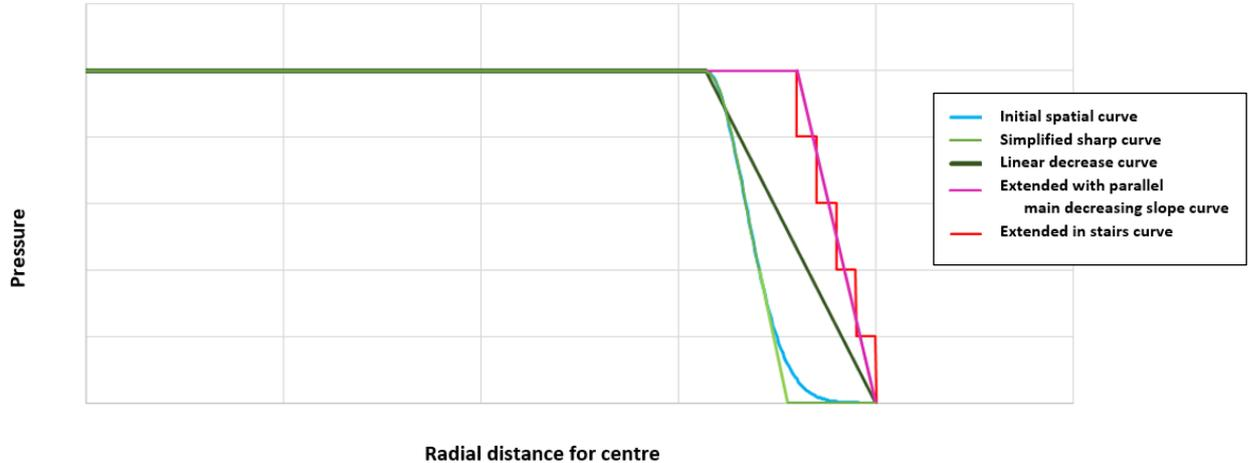
Fig.6: Different spatial pressure loadings
