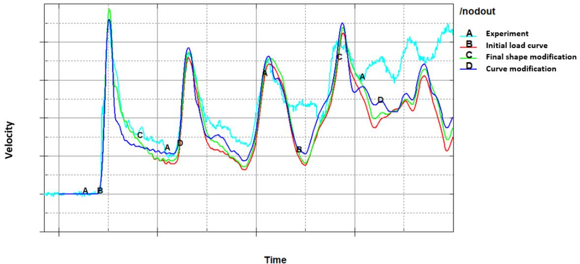
Fig.5: Back face velocity versus time depending on different pressure loadings
