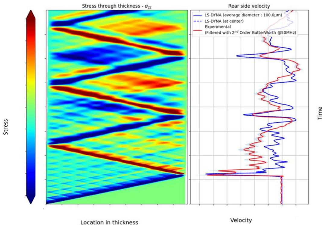
Fig.11: XT Diagram for the quarter 3D model representing laser impact on CFRP composite
