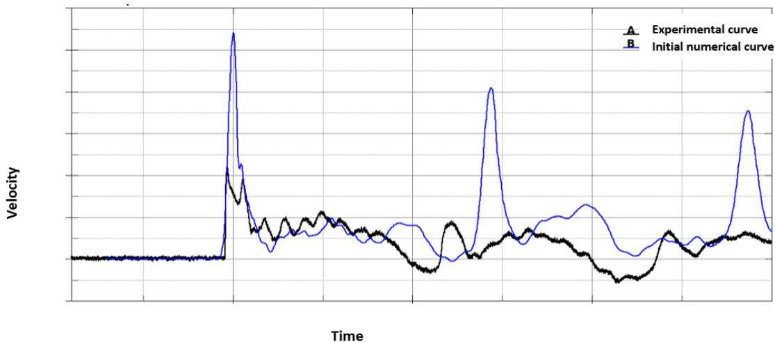
Fig.8: Comparison of back face velocities between experimental and numerical results on a composite plate
