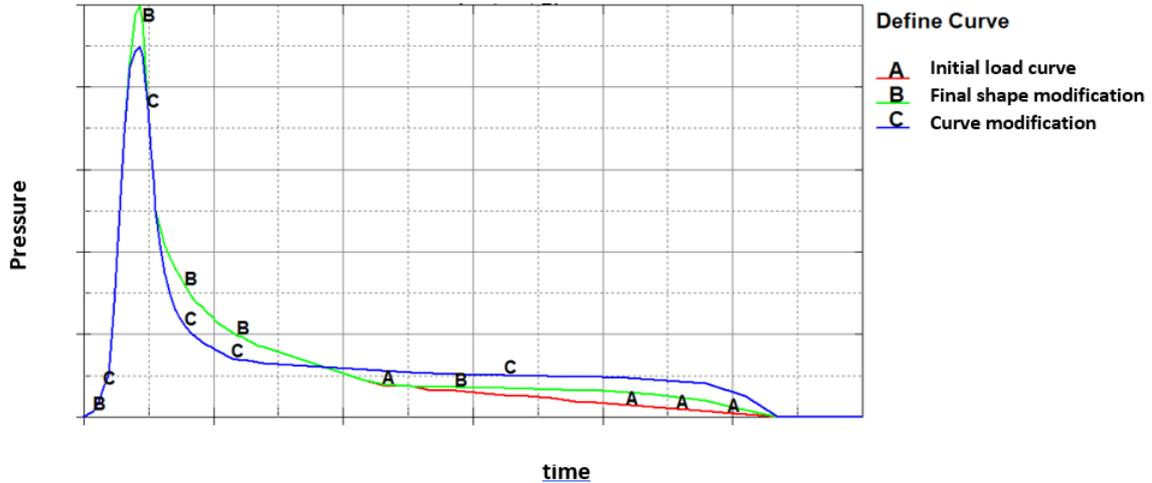
Fig.4: Different temporal pressure loadings
