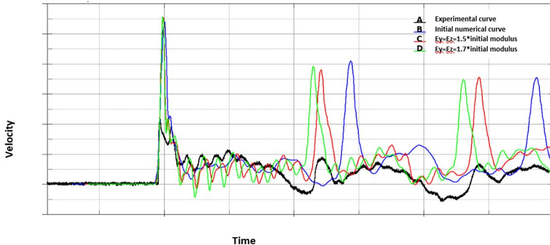
Fig.9: Back face velocity evolution depending on the composite transversal modulus value
