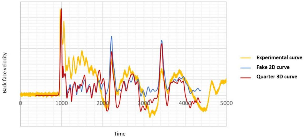
Fig.10: Comparison of back face velocities between experimental and numerical results depending on the modelling strategy
