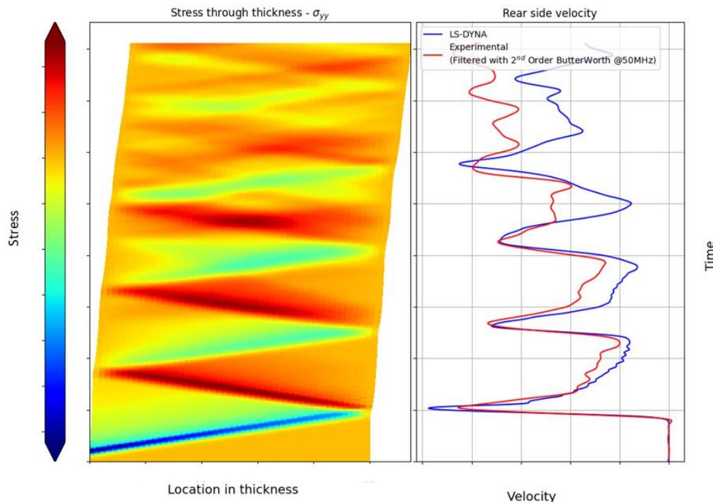
Fig.3: XT Diagram for the 2D axisymmetric model representing laser impact on Aluminium 2024
