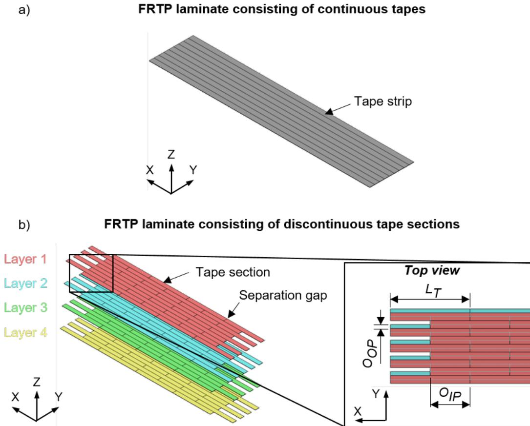
Fig.2: Comparison of the structure of an F RTP laminate with a) continuous tapes and b) discontinuous tape sections.
