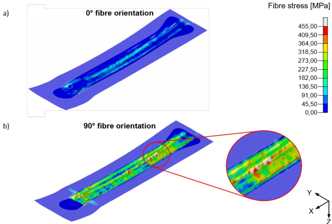
Fig.6: Stress distribution of the fibres considering a) the layers with 0° fibre orientation and b) with 90° fibre orientation.
