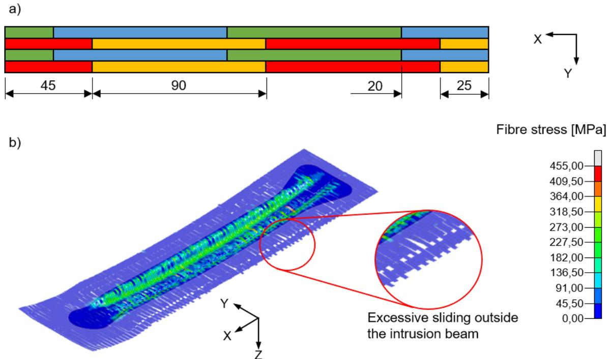
Fig.7: a) Layer structure of the FRTP using discontinuous tape sections; b) Stress distribution of the layer, consisting of discontinuous tape sections.
