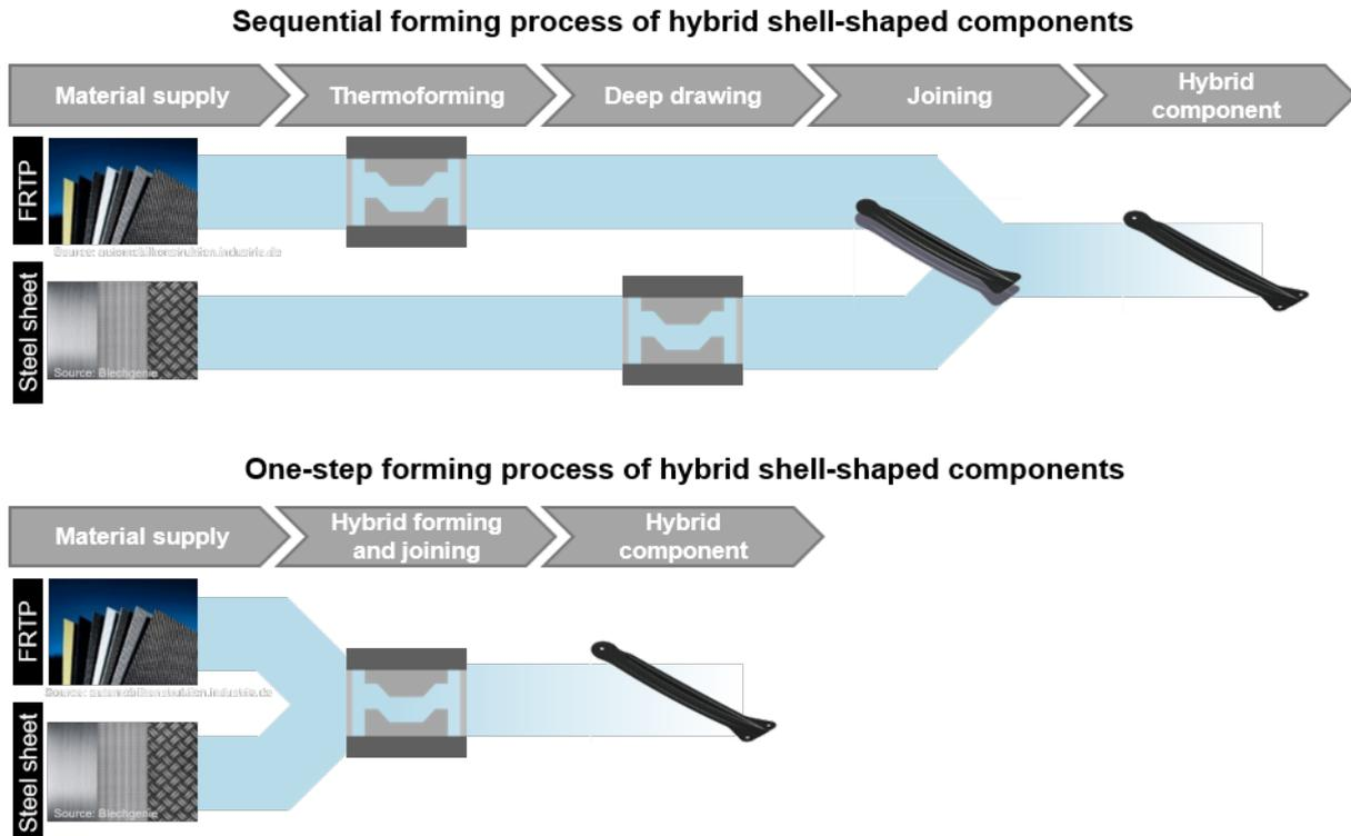
Fig. 1: Comparison of the sequential and one-step forming process for the production of hybrid shell-shaped components.
