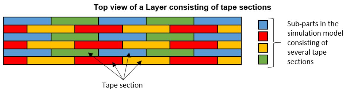
Fig.4: A layer of FRTP laminate using discontinuous tape sections. The layer composed of four sub-parts consisting of several tape sections that are not in direct contact.
