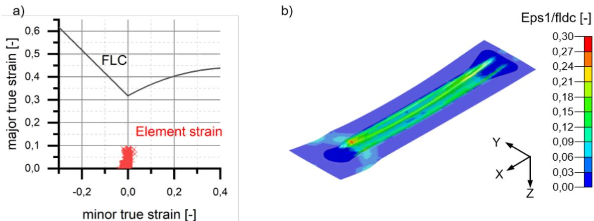
Fig.5: a) Main and secondary strain of the elements of the steel sheet as well as the forming limit curve; b) Strains in the formed steel sheet.
