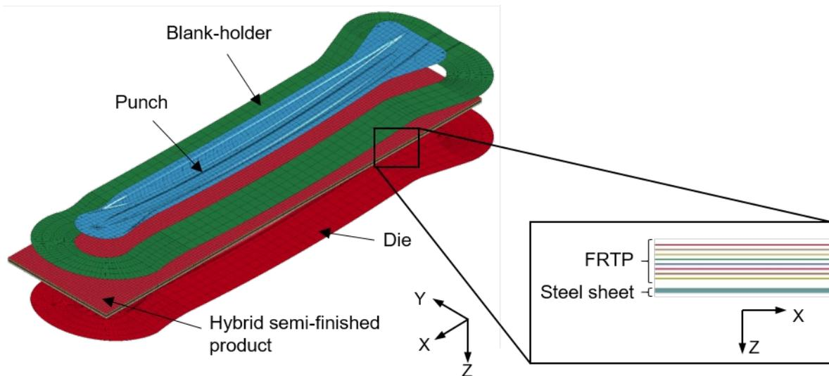
Fig.3: Structure of the simulation model.
