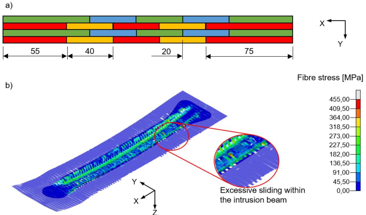
Fig.8: a) Revised structure of the FRTP using discontinuous tape sections; b) Stress distribution of the revised layer structure, consisting of discontinuous tape sections.
