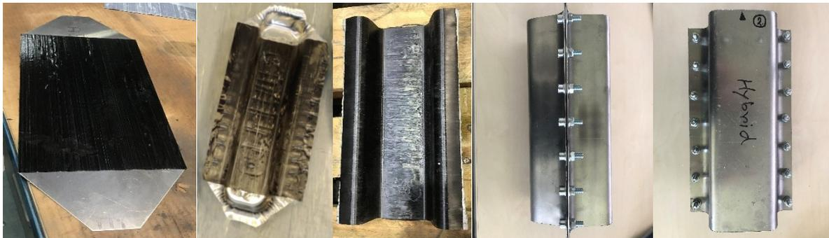
Fig.1: Manufacturing steps (from left to right) of the hybrid generic crash element.
