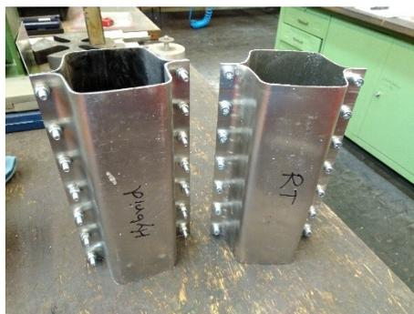
Fig.2: Generic crash element: (left) aluminum-CFRP hybrid component, (right) aluminum component.
