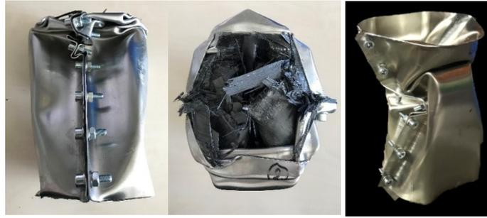
Fig.3: After crush test: (left & middle) aluminum-CFRP hybrid component, (right) aluminum component.
