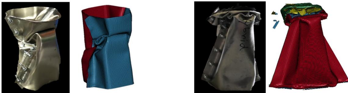
Fig.9: Deformed shape (simulation and experiment) after crushing: (left) aluminum profile; (right) aluminum-CFRP hybrid profile.
