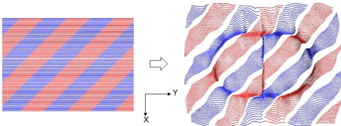
Fig.12: Initial and final deformation behavior of 90 degree angle fiber orientation layer
