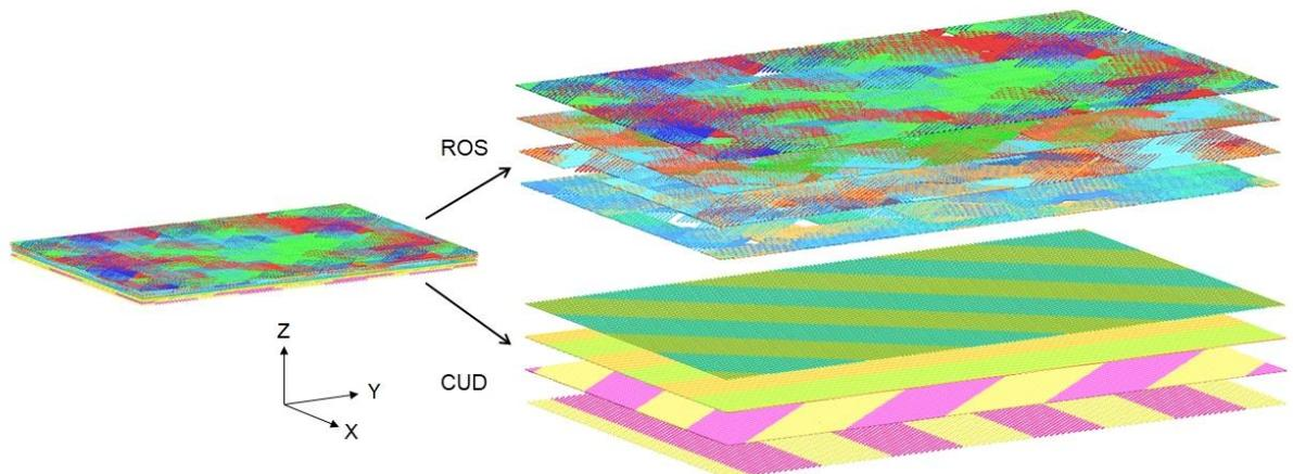
Fig.6: Hybrid lay-up fiber model: upper layers ROS type and lower layers CUD type
