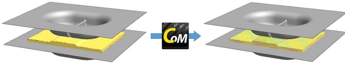
Fig.13: Compression molding simulation model using convex shaped matrix resin model
