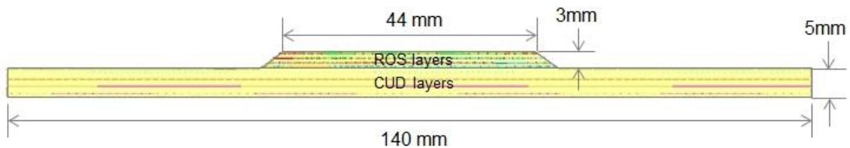
Fig.14: Dimensions of convex shape matrix resin model and fiber orientations
