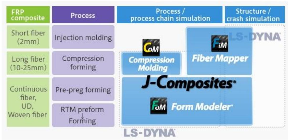
Fig.1: The set of tools in J-Composites
