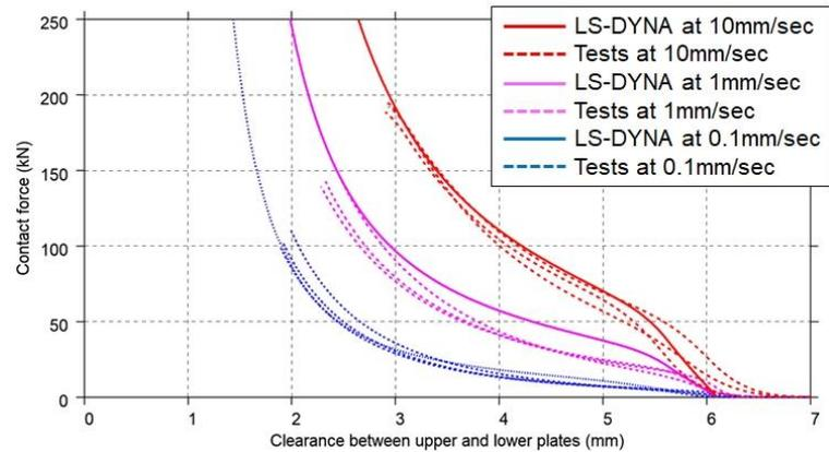
Fig.9: Squeeze flow test results of LS-DYNA and tests
