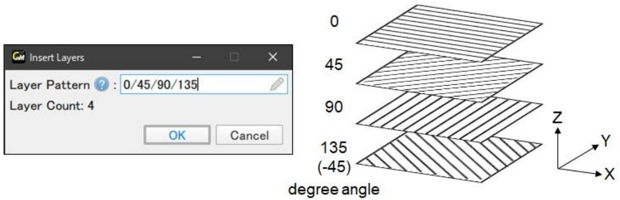
Fig.4: Input panel to enter layer pattern
