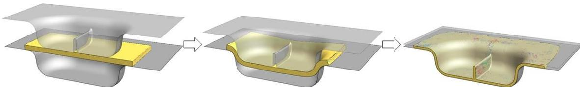
Fig.11: Compression molding simulation result of hybrid lay-up composite model
