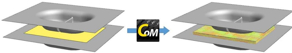
Fig.10: Compression molding simulation model using hybrid lay-up composite
