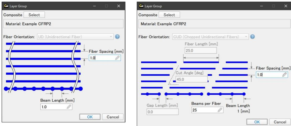
Fig.3: Input panels to define UD (left) and CUD (right)
