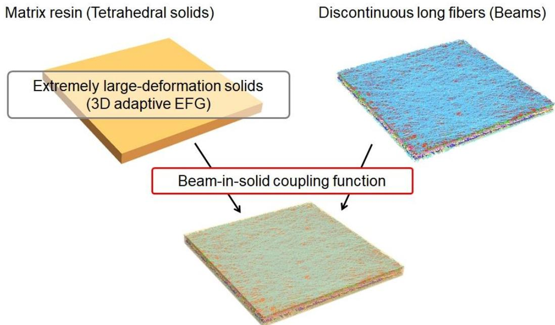
Fig.2: Matrix resin by tetrahedral solids and discontinuous long fibers modelled by beams
