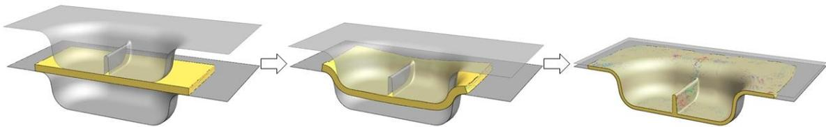
Fig.11: Compression molding simulation result of hybrid lay-up composite model
