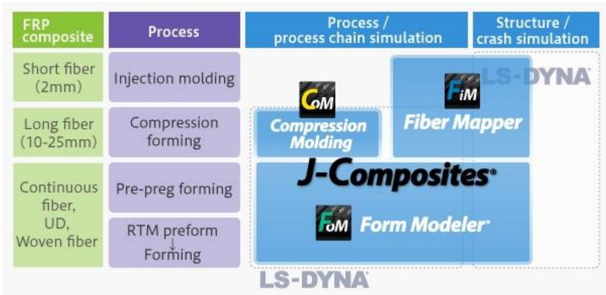
Fig.1: The set of tools in J-Composites
