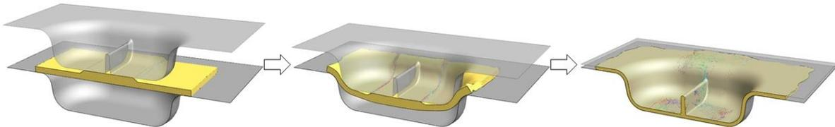
Fig.15: Compression molding simulation result of convex shaped matrix resin model
